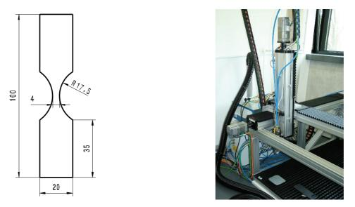
Fig. 3 Shape and dimensions of testing sample (left) and lay-out of the whole laser cutting workplace (right)
