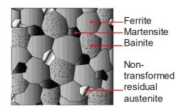
cutting method and its character has a very important influence on the subsequent work piece plastic properties [2]. That is why this paper deals with the influence of cutting technologies on the cyclic fatigue of so-called TRIP steel (structure - **Fig. 1**) cause this steel is able to reveal strengthening during impact and thus to absorb part of impact energy.
