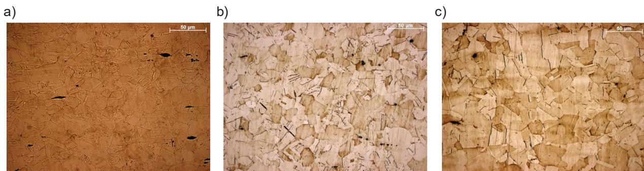
**Fig. 5** Austenitic structures of high manganese X13MnSiAlNbTi25-3-3 TWIP-type steel obtained after four-stage hot compression test followed by heat treatment at: a) temperature 850 $^{\circ}\text{C}$  for 300s; b) temperature 950  $^{\circ}\text{C}$  for 900 s; c) temperature 1000  $^{\circ}\text{C}$  for 900 s
