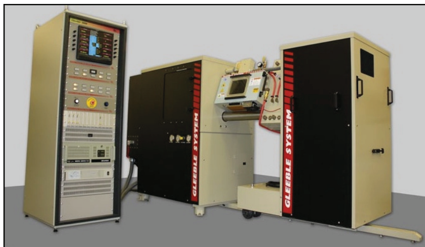
Fig. 1 The simulator metallurgical processes Gleeble 3800
