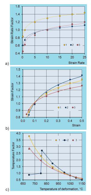
**Fig. 1** Variation factors influence strain rate (a), strain (b) and temperature (c): 1, 2, 3 - by the formulas (6), (7) and (8) respectively
