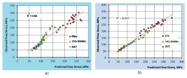
**Fig. 3** Charts of compliance of Predicted and Observed Flow Stress: a) calculated using the formula (9); b) calculated using the formula (14)
