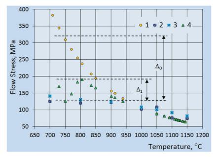
**Fig. 2** The dependence of Flow Stress on temperature for rolled sheet steel X70: 1, 2, 3 - calculated using the formula (6), (7) and (8); 4 - calculated by the formula (9)
