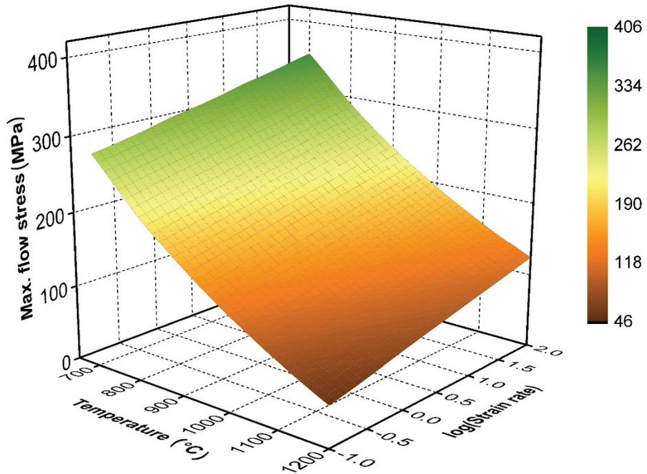
Fig. 3 3D-graph of maximum flow stress of the steel P355NH depending on temperature and strain rate
