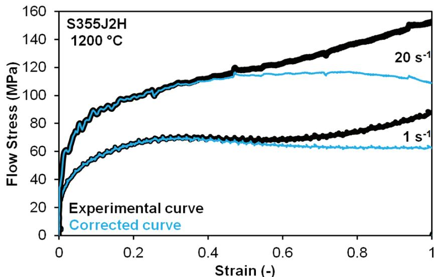
**Fig. 1** Flow stress curve correction
