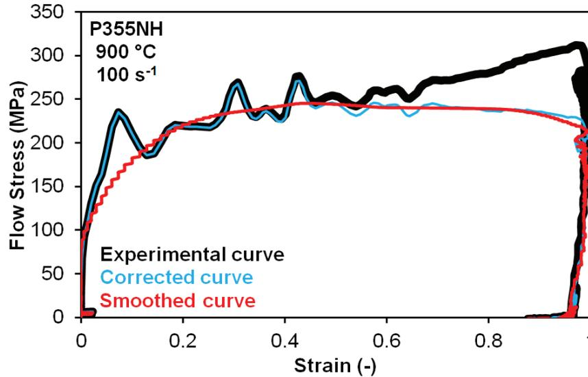
Fig. 2 Flow stress curve smoothing
