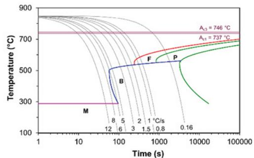
**Fig. 4** CCT diagram of steel 51CrV4 constructed by using the software QTSteel 3.2.
