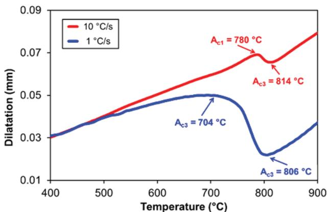
**Fig. 1** Determination of transformations temperatures
