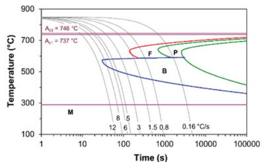
**Fig. 8** DCCT diagram of steel 51CrV4 constructed by using the software QTSteel
