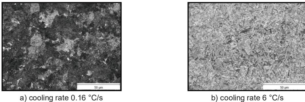
**Fig. 6** Examples of microstructure of the samples subjected to dilatometric tests (without deformation)
