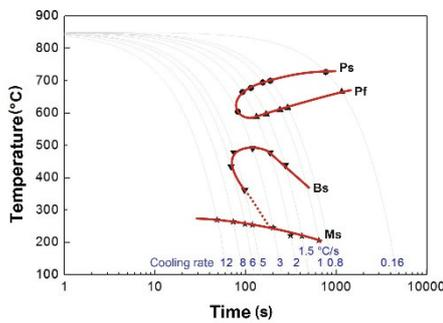
**Fig. 3** CCT diagram of steel 51CrV4
