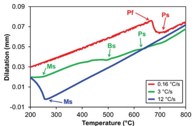
**Fig. 2** Dilatation curves for cooling of the spring steel 51CrV4 (without of preceding deformation)
