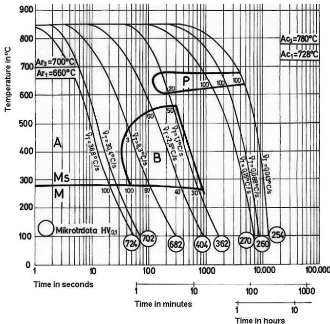
**Fig. 5** CCT diagram of equivalent steel 50CrV4 [16]
