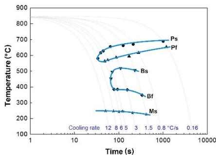
**Fig. 7** DCCT diagram of steel 51CrV4
