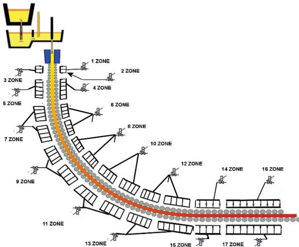
**Fig. 3** Diagram 17 cooling zones slab caster (Type C)
