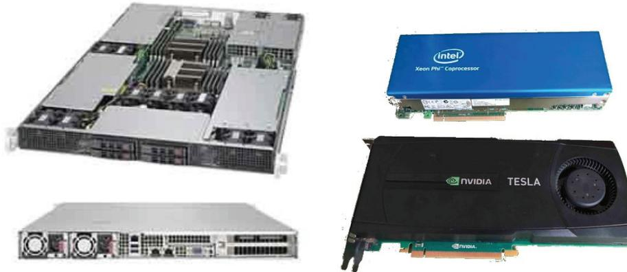
Fig. 5 Example of server hardware and computational accelerator cards [12]
