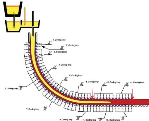
**Fig. 1** Diagram 9 cooling zones slab caster (Type A) **Fig. 2** Diagram 13 cooling zones slab caster (Type B)
