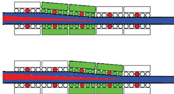
**Fig. 4** How it works softreduction
