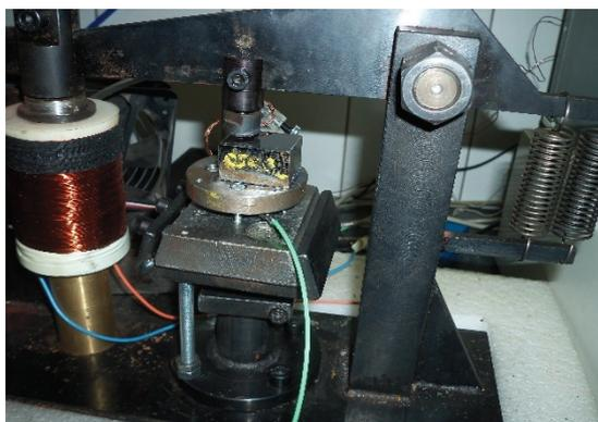
**Fig. 2** Electronically controlled impact tester
