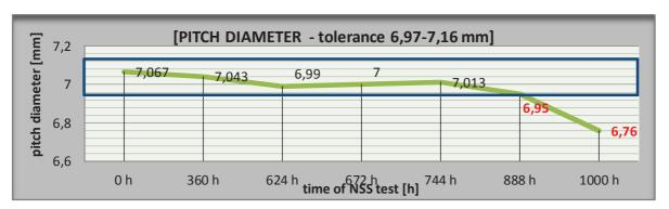
Fig. 4 Pitch diameter change during the corrosion process
