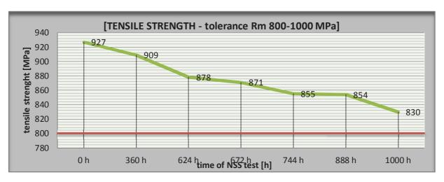
Fig. 2 Influence of corrosion on the tensile strength change
