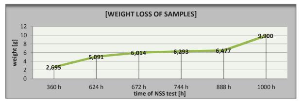
Fig. 3 Weight change during the corrosion process
