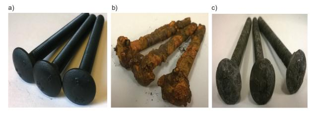
**Fig. 1** The screws M8x80 appearance: a) - before corrosion test, b) - after corrosion test, c)- after cleaning the surface - removal of corrosion products
