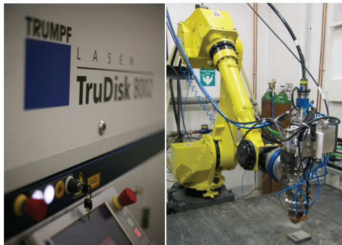
Fig. 1 The cladding system
