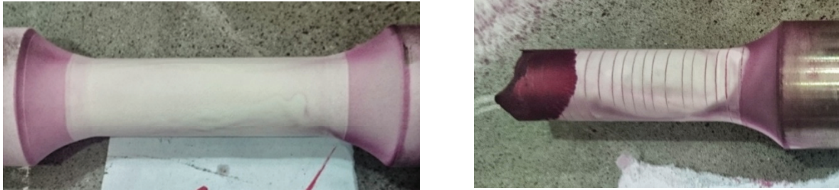
Fig. 3 Capillary testing of \text{Cr}_3\text{C}_2\text{-NiCr} coating at 20 °C (Left - sample with load under the fatigue life limit, right - sample above fatigue life limit)
