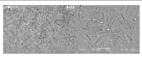
**Fig. 5** Left image: light micrograph of a longitudinal sample ref.U1: martensitic and bainitic microstructure. Right image: presence of carbides
