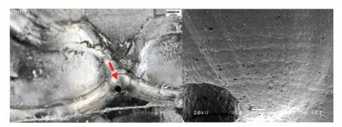
Fig. 4 SEM micrograph. Presence of marks attributed to an erosion process
