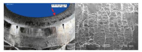
Fig. 2 SEM micrograph of cracks net and oxides on ref. U1
