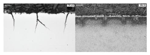
Fig. 3 Light micrographs of ref.U1. Left image: presence of triangular cracks and oxides filling them. Right image: etch condition, presence of a nitrided layer
