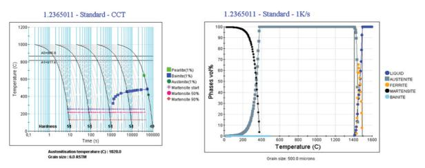
Fig. 6 CCT-diagrams and phase stability diagram of 1.2365 (JMatPro Calculations)
