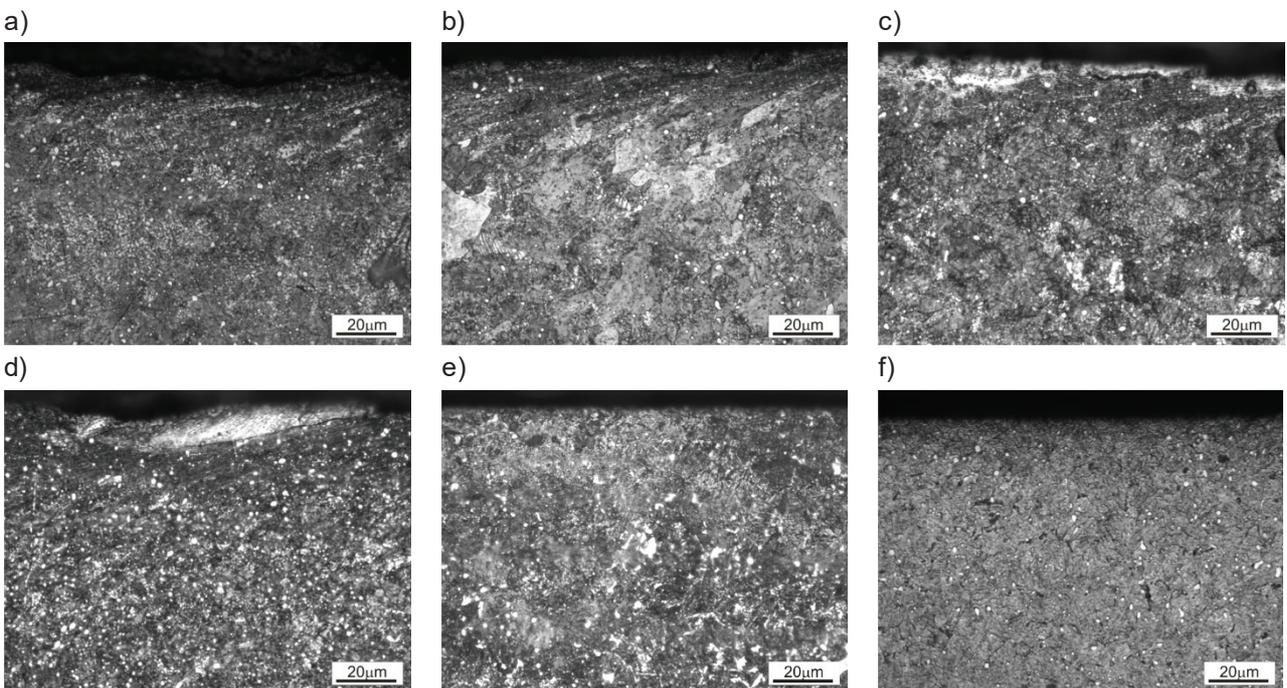
**Fig. 4** Microstructure of the samples in cross section cooled with the cooling rate of: a) 0.076 °C/s; b) 0.24 °C/s; c) 0.83 °C/s; d) 2.17 °C/s; e) 6.5 °C/s; f) 21.4 °C/s
