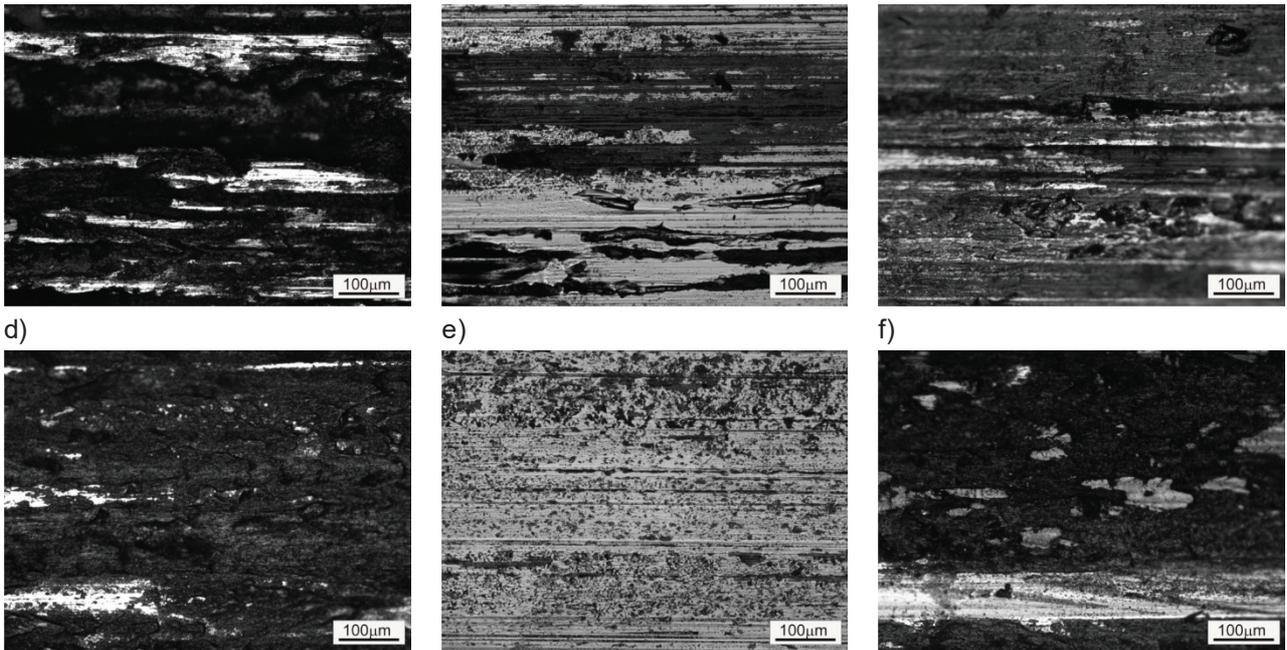
**Fig. 3** The image of the wear surface of the samples cooled with the cooling rate of: a) 0.076 °C/s; b) 0.24 °C/s; c) 0.83 °C/s; d) 2.17 °C/s; e) 6.5 °C/s; f) 21.4 °C/s
