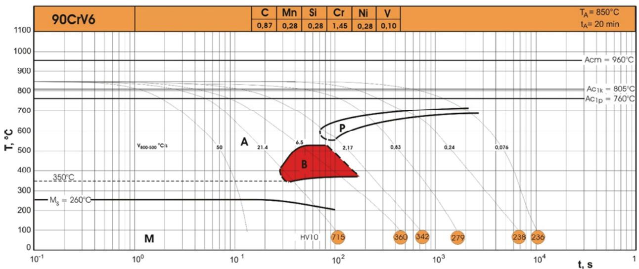
**Fig. 1** CCT diagram of 90CrV6 steel [7]
