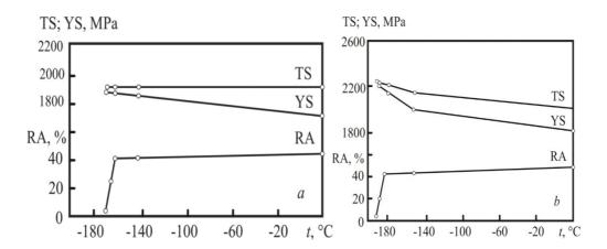
**Fig. 3** Temperature dependences of mechanical properties of steel 0.4CCrNi: treatment by variant 1(a); treatment by variant 3 (TMP) (b)
