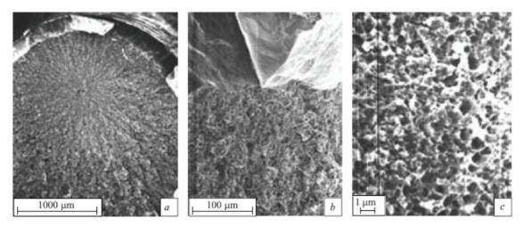
Fig. 4 Fracture surfaces (t<sub>test</sub> = - 196 °C) of steel 0.4CCrNi after TMP (variant 3)
