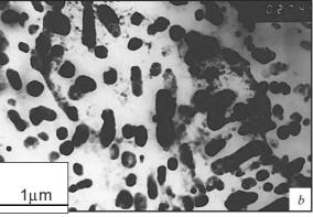
**Fig. 1** Structure of steel 0.4CCrNi after annealing for lamellar (a) and granular (b) pearlite
