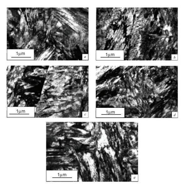
**Fig. 2** Structure of steel 0.4CCrNi after: quenching of non-deformed billets from furnace and induction heating respectively (a, b); cold rolling before quenching from induction heating (c); cold rolling and annealing respectively at 500 and 600 °C before quenching and induction heating (d, e)
