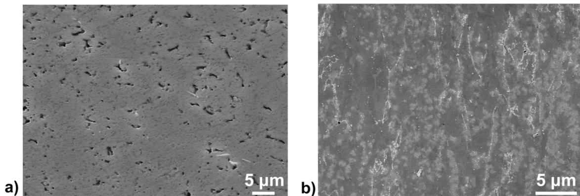
**Fig. 1** Microstructures of swaged sample (a), sample after HPT (b)
