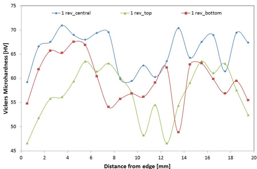
**Fig. 3** Microhardness values for HPT processed specimens
