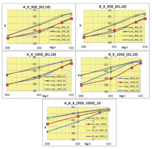
**Fig. 5** Avrami curves for various samples (A\_1183 (12 % Mn); B\_1184 (22 % Mn) and temperatures and strain rates
