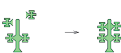
Fig. 1 Assembly of individual wax models into tree
