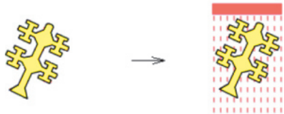
Fig. 3 Sanding - making a final surface of layer
