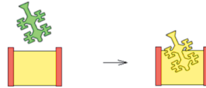
Fig. 2 Trees dipping into a ceramic slurry
