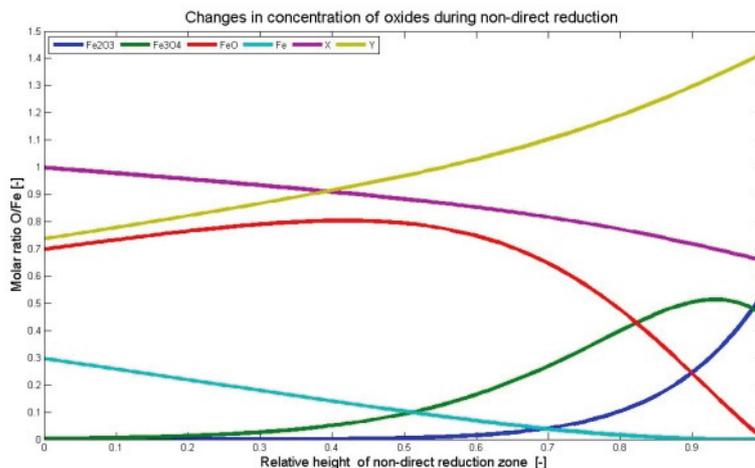
**Fig. 3** Reduction process of sample 2
