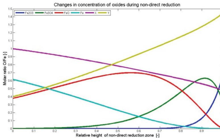
**Fig. 2** Reduction process of sample 1
