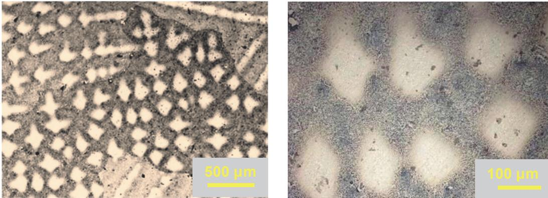
**Fig. 3** Microstructure of the Ni-8Al-12.5Mo alloy (sample A1-20), directed state: 20 mm/h, cross section
