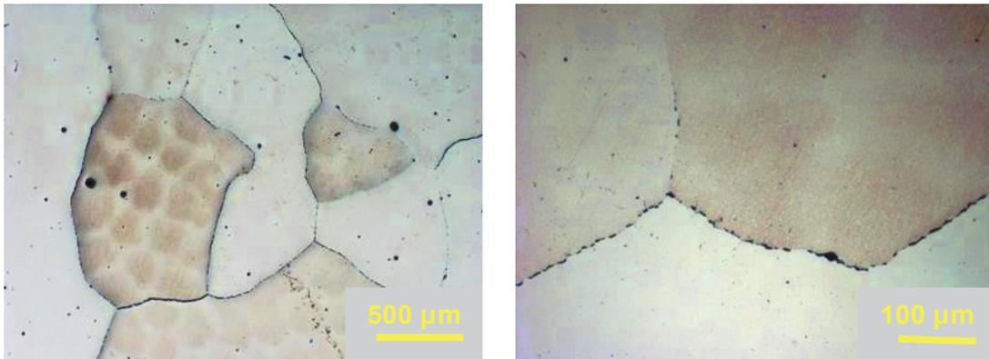
**Fig. 7** Microstructure of the Ni-8Al-9.5Mo alloy (sample C1-20), directed state: 20 mm/h, cross section
