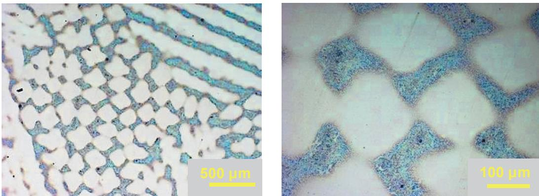
**Fig. 5** Microstructure of the Ni-8Al-11Mo alloy (sample B1-20), directed state: 20 mm/h, cross section
