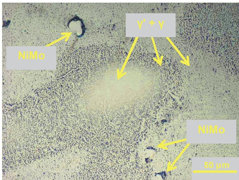
**Fig. 8** Sample No. A1-50, Mo rich alloy - detail of structure
