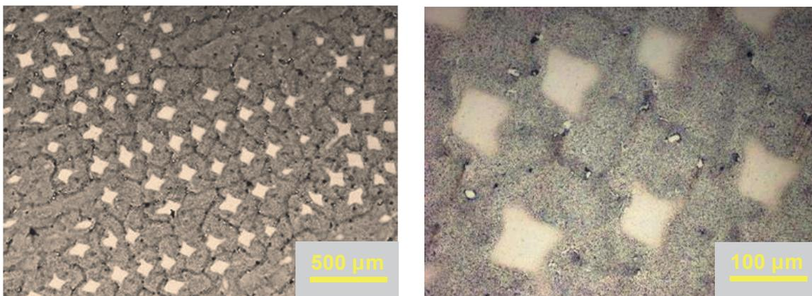
**Fig. 2** Microstructure of the Ni-8Al-12.5Mo alloy (sample A1-50), directed state: 50 mm/h, cross section
