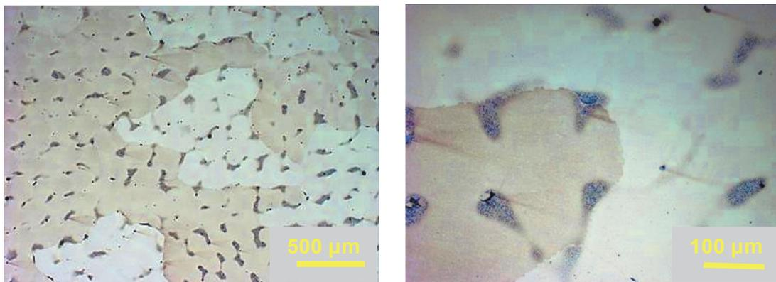
**Fig. 6** Microstructure of the Ni-8Al-9.5Mo alloy (sample C1-50), directed state: 50 mm/h, cross section
