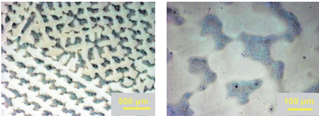
**Fig. 4** Microstructure of the Ni-8Al-11Mo alloy (sample B1-50), directed state: 50 mm/h, cross section
