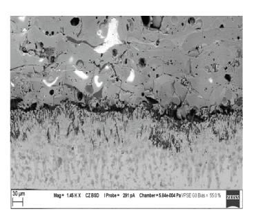
Fig. 4 Ceramic (Eucor) coating on Fe<sub>2</sub>B interlayer
