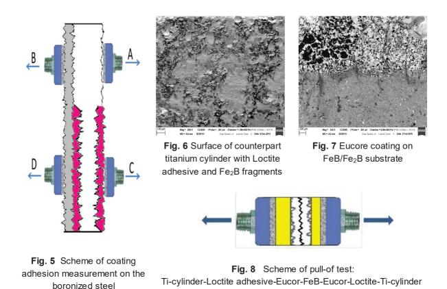
It follows from the above, that strength of the eucor-steel joint is higher than tensile strength of eucor ceramics. Relation between this strength and impact on its value by primary roughness in the joint /on the interface/ has not been in this case measured quantitatively but proved logic and followed also from our similar measurements performed for example on phosphate systems [9].
