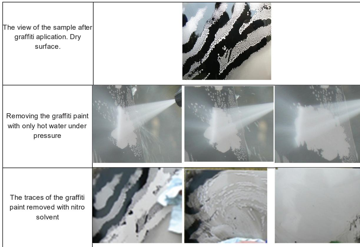
**Fig. 1** Steps in removing spray paint from anti-graffiti coatings
