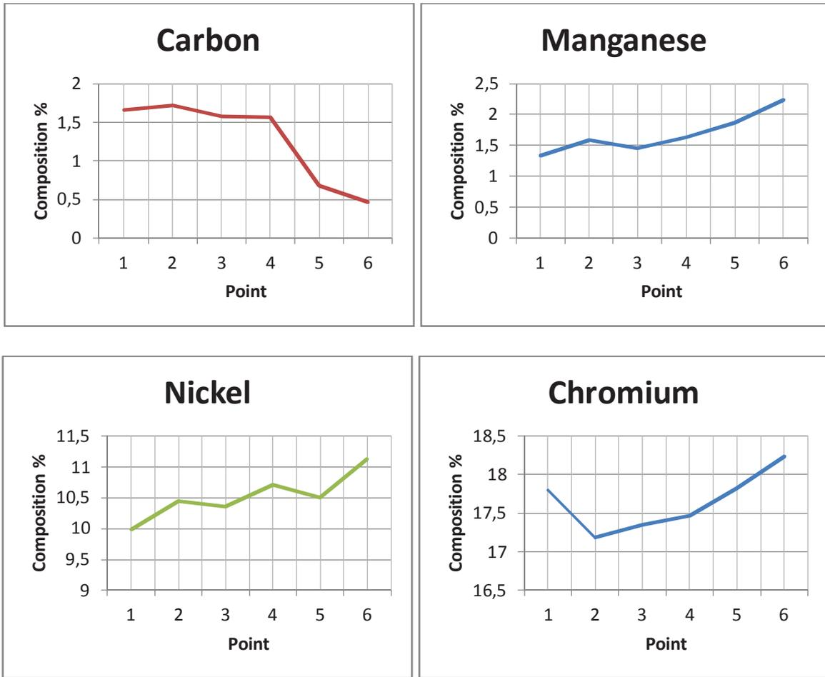
**Fig. 4** Chemical composition variation in points from external wall (point 1) to the internal wall (point 6)
