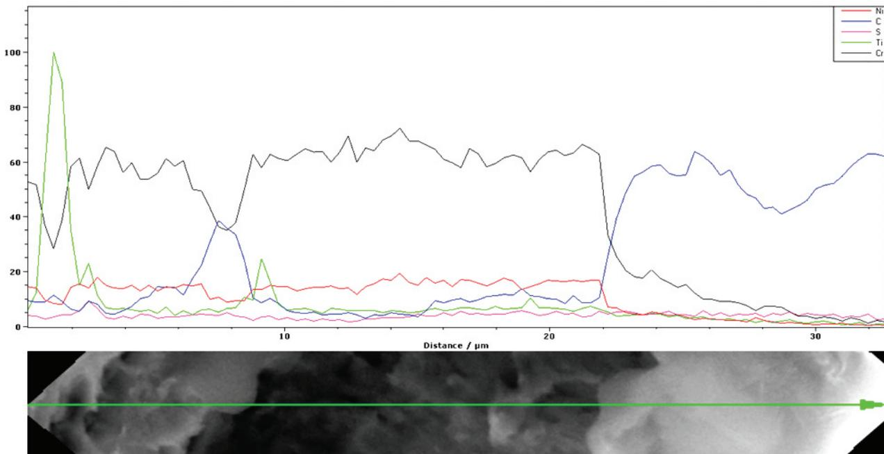
**Fig. 5** EDAX of the chemical composition at grain boundaries
