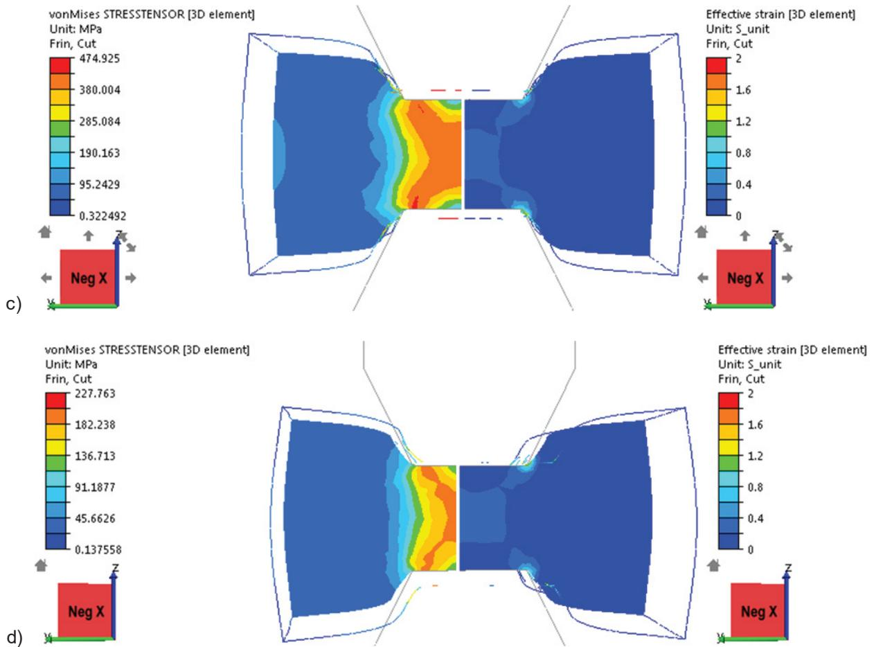
**Fig. 4** The value of the intensity of stresses and effective strains for: a) variant 1, b) variant 2, c) variant 3, and d) variant 4
