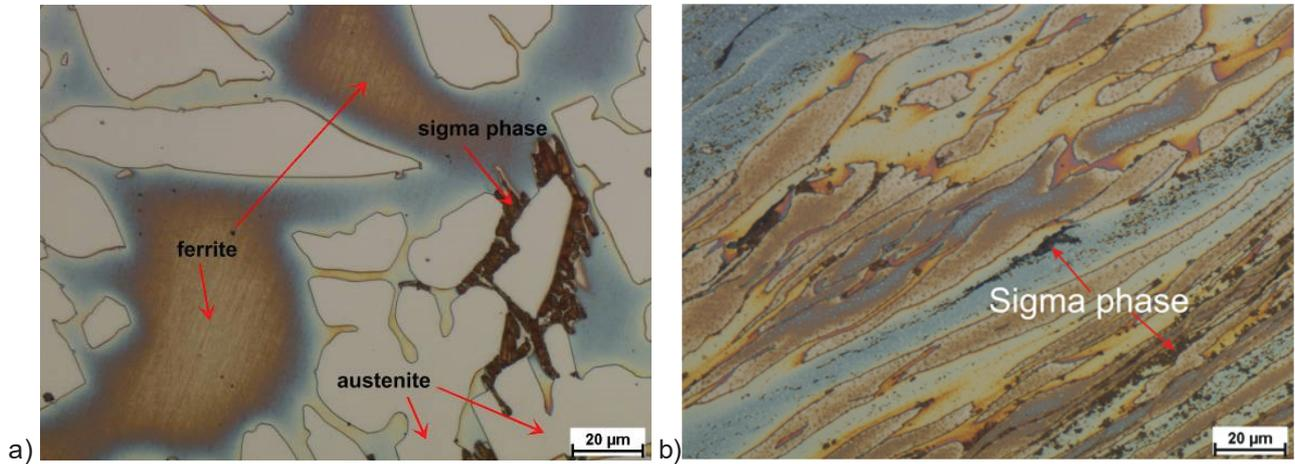
**Fig. 3** Example of samples microstructures. a) Sample not deformed., b) Sample deformed sample deformed at 950 °C with strain rate 1.0 and  $\epsilon=1.3$
