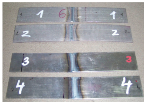
Fig. 1 Welded samples (1, 2-after 6xDRECE, 3, 4-IS)
