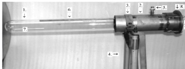
**Fig. 1** Reactor used in corrosion resistance tests of valve steels in hot flux of exhaust gases from a combustion engine: 1 - the glass tube of the reactor, 2 - steel housing, 3 - grip, 4 - pedestal, 5 - connector pipe, 6 - pipe delivering the combustion gases to reactor, 7 - oxidation area of samples, 8 - collar, 9 - combustion outlet
