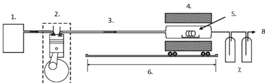
**Fig. 2** The scheme of setup used in corrosion tests: 1- fuel tank, 2 - combustion engine, 3 - delivering pipe of combustion gas, 4 - furnace, 5 - reactor with samples, 6 - range of funeral movement, 7 - combustion bulbs, 8 - combustion outlet
