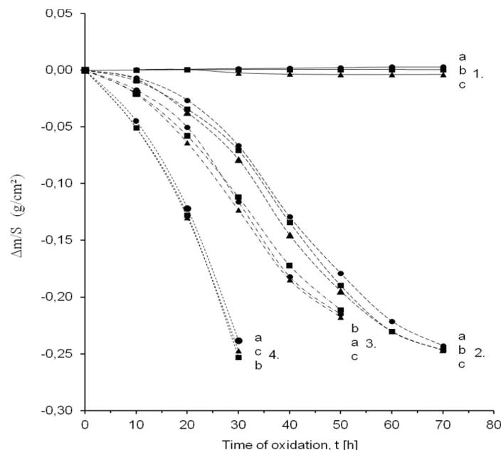
**Fig. 3** Corrosion resistance of the valve steels 1 - X33CrNiMnN23-8, 2 - X50CrMnNiNbN21-9, 3 - X53CrMnNiN20-8 and 4 - X55CrMnNiN20-8 in combustion gases of petrol with: a - 5 %, b - 10 % and c - 50 % ethanol additive [v/v]. The samples were oxidized under the conditions of cyclic thermal shocks at the temperature of 1173 K
