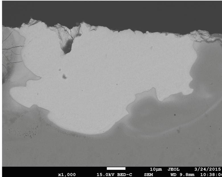
**Fig. 3** SEM image of crosssection of the single crater on alloyed surface layer after the ESD process (U = 25 V) mag. x1000
