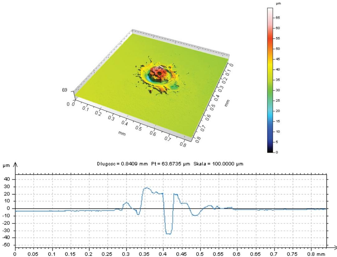
**Fig. 1** View of 3D single crater on machined surface made by Talysurf CCI Lite -- Taylor Hobson scanning profilometer type
