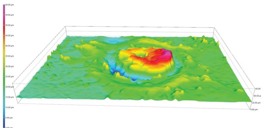
**Fig. 2** View of 3D single crater topography on alloying surface made by Nikon Eclipse MA 200
