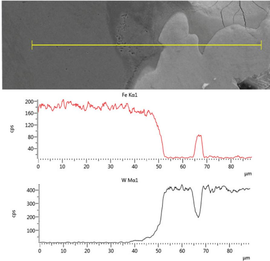
**Fig. 5** X-ray line scan of the superficial layer after the ESD process ( $U = 25 V$ ) using a tungsten electrode - a; chemical elements distribution in the sub-surface layer - b;
