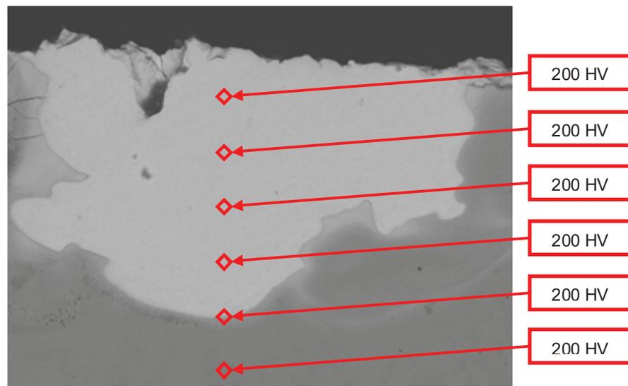
**Fig. 4** Microhardness distribution in a crosssection of the surface layer after the ESD process (U = 25 V), steel (C 45)
