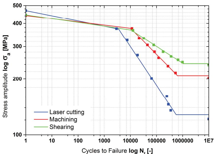
**Fig. 8** Wöhler's curves of TRIP steel RA-K 40/70 for different material cutting technologies
