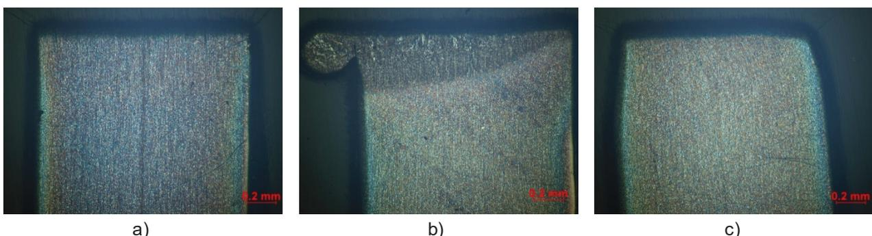
**Fig. 4** Shapes of cut edges for milling (a), laser cutting (b), shearing (c).
