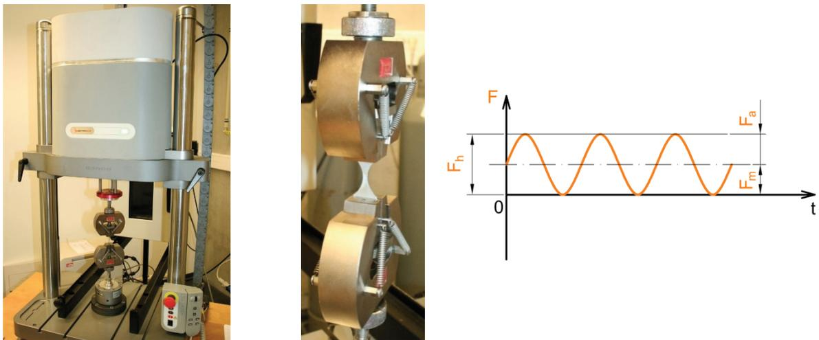
**Fig. 5** Machine for cyclic tests Instron E3000 and chosen loading cycle
