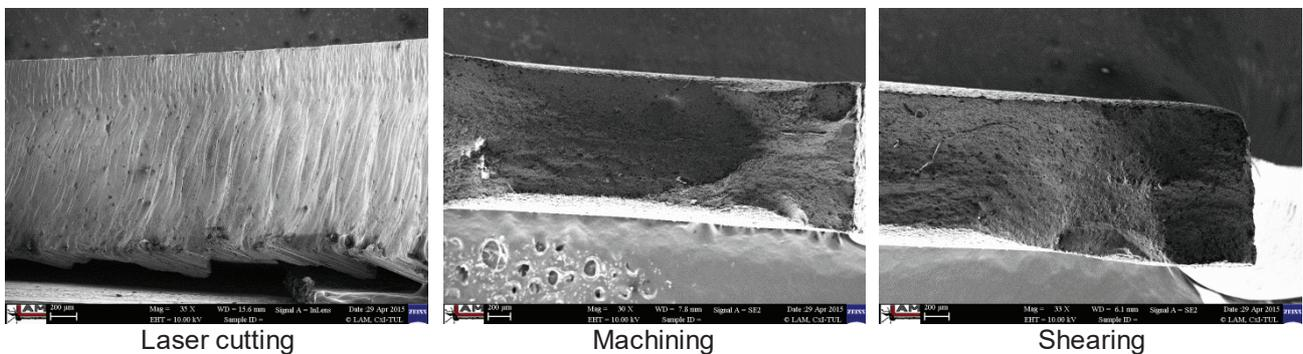
Fig. 7 Images of fatigue failure surfaces loaded by transient cycle with amplitude of stress 325 MPa
