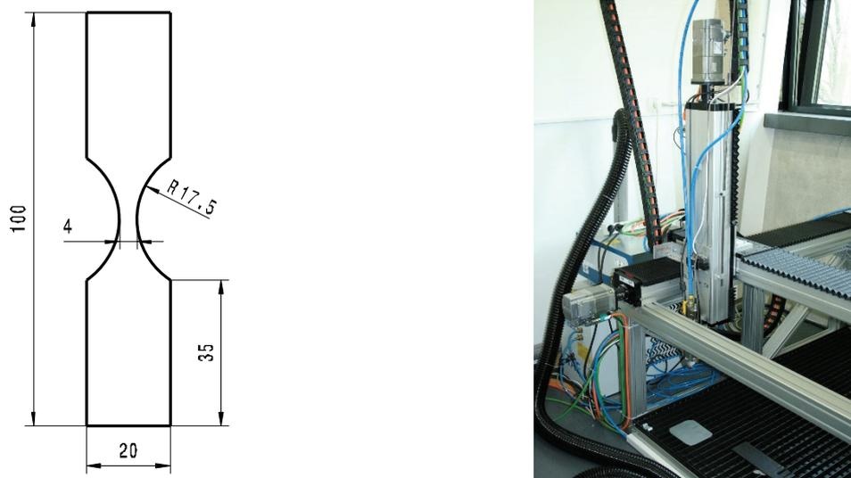
**Fig. 3** Shape and dimensions of testing sample (left) and lay-out of the whole laser cutting workplace (right)
