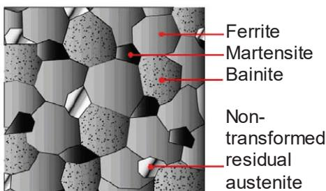
cutting method and its character has a very important influence on the subsequent work piece plastic properties [2]. That is why this paper deals with the influence of cutting technologies on the cyclic fatigue of so-called TRIP steel (structure - **Fig. 1**) cause this steel is able to reveal strengthening during impact and thus to absorb part of impact energy.
