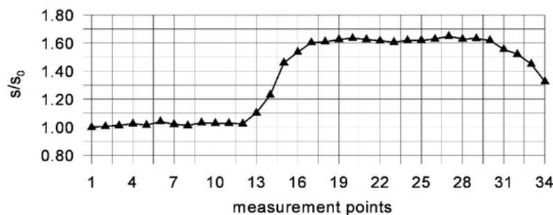
**Fig. 6** The wall thickness distribution in the longitudinal section of the rolled reducing tube from MT1020 steel at  $s_0/D=0.09$  and  $K=1.46$  ratios, where: a) spacing of measurement points, b) the wall thickness distribution graph
