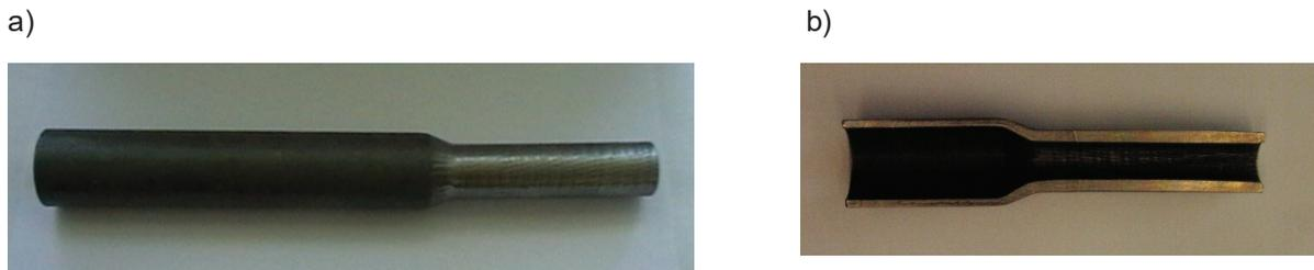
**Fig. 4** Examples of experimentally rolled MT1020 steel reducing tubes at  $s_0/D=0.09$  and  $K=1.46$  ratios, where: a) reducing tube, b) longitudinal section of the reducing tube
