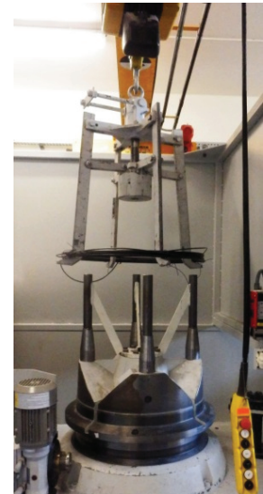
Fig. 3 Lifting the coil holder from the drawing block
