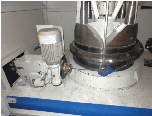
Fig. 1 KOCH KGT 25 - E wire-drawing machine: rotating die holder and drawing block during wire introduction by the wire pulling-in dog
