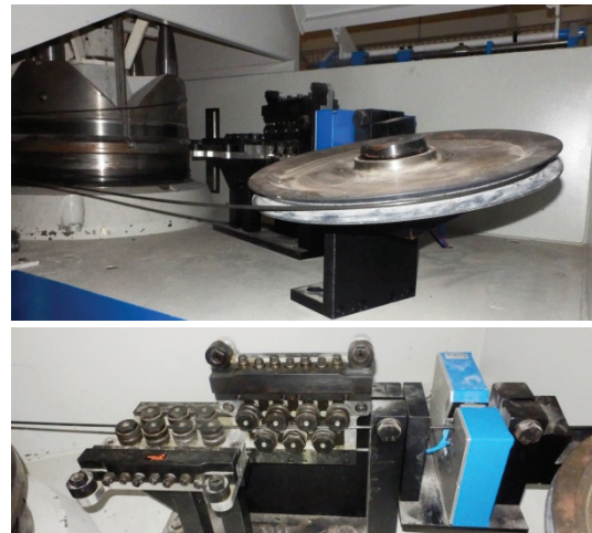
Fig. 2 top: transfer pulley, bottom: laser measurement of dimensions and wire straightener
