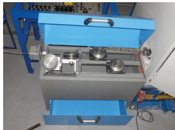
Fig. 5 Roller descaler with spiral wire brushes
