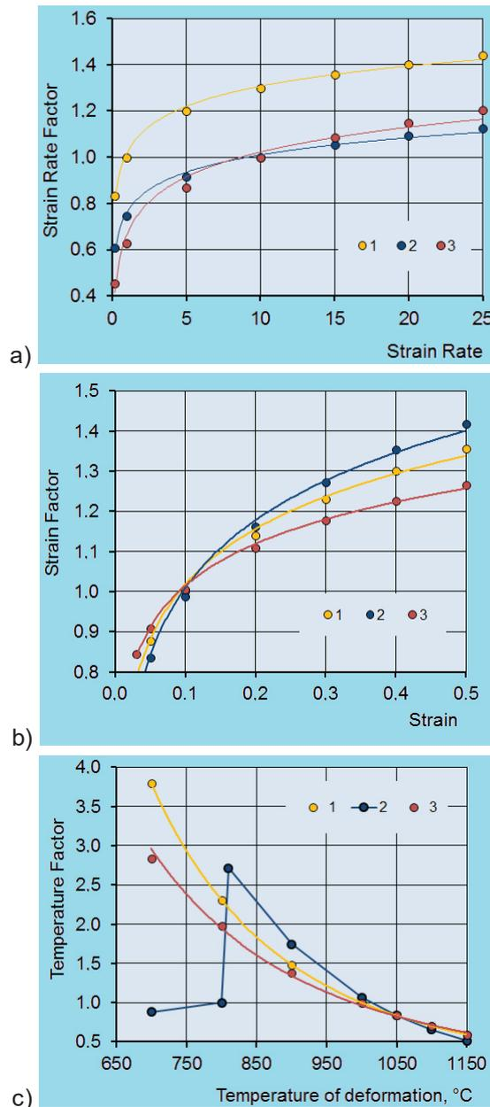
Fig. 1 Variation factors influence strain rate (a), strain (b) and temperature (c): 1, 2, 3 - by the formulas (6), (7) and (8) respectively
