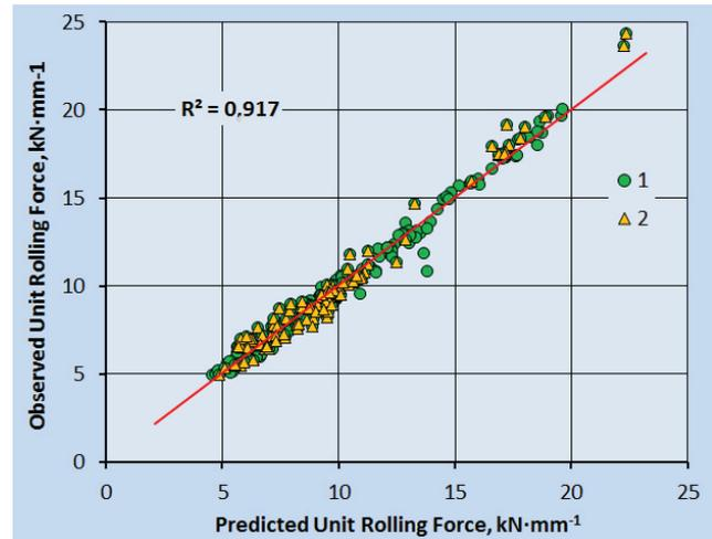
**Fig. 4** Charts of compliance of Predicted and Observed Unit Rolling Force:
