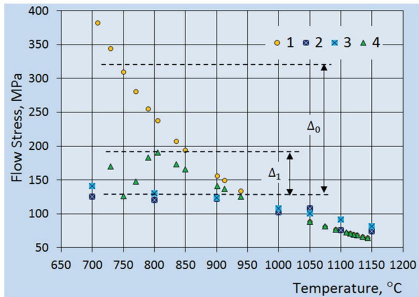
**Fig. 2** The dependence of Flow Stress on temperature for rolled sheet steel X70:
