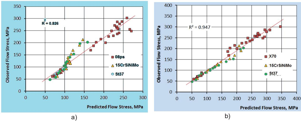
**Fig. 3** Charts of compliance of Predicted and Observed Flow Stress:
