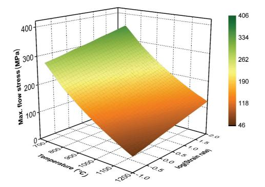
Fig. 3 3D-graph of maximum flow stress of the steel P355NH depending on temperature and strain rate
