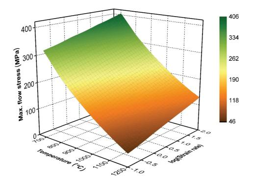
Fig. 4 3D-graph of maximum flow stress of the steel S355J2H depending on temperature and strain rate
