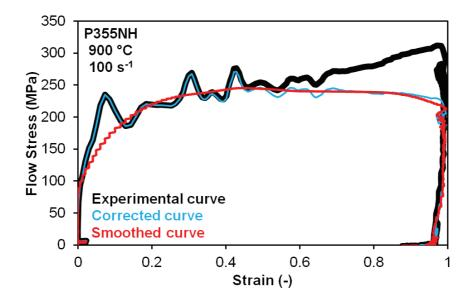
Fig. 2 Flow stress curve smoothing
