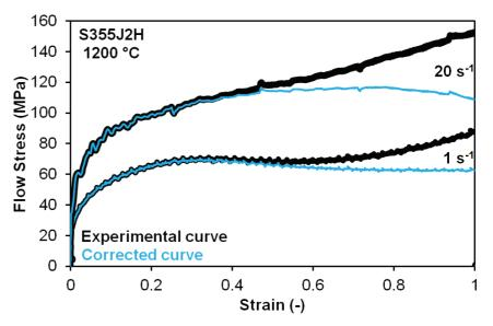
Fig. 1 Flow stress curve correction
