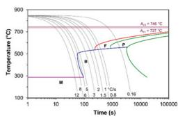
Fig. 4 CCT diagram of steel 51CrV4 constructed by using the software QTSteel 3.2.
