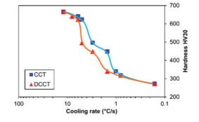
Fig. 10 Comparison of CCT and DCCT disintegration diagrams determined by dilatometry of steel 51CrV4
