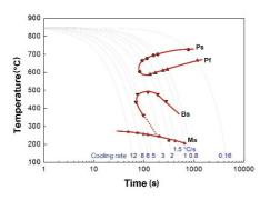
Fig. 3 CCT diagram of steel 51CrV4
