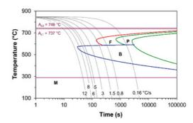
Fig. 8 DCCT diagram of steel 51CrV4 constructed by using the software QTSteel
