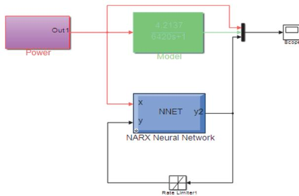
**Fig. 3** Test of ANN using model of plant
