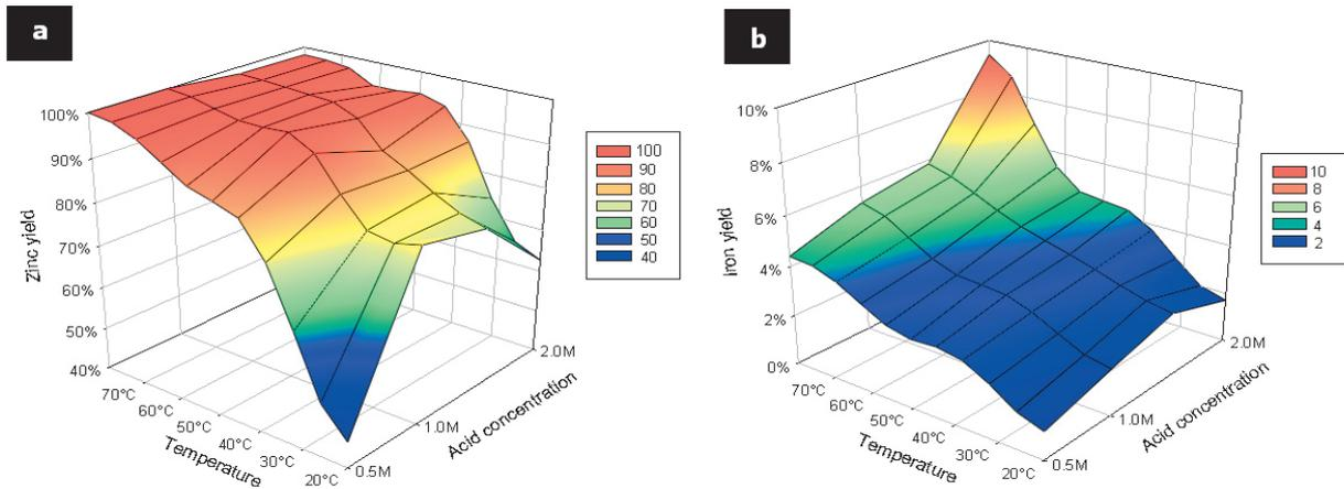
**Fig. 4** Zinc (a) and iron (b) leached illustrated as a function of temperature and acid concentration in 15<sup>th</sup> minute of experiment
