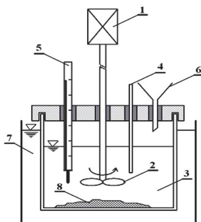
**Fig. 1** Leaching apparatus [11]
