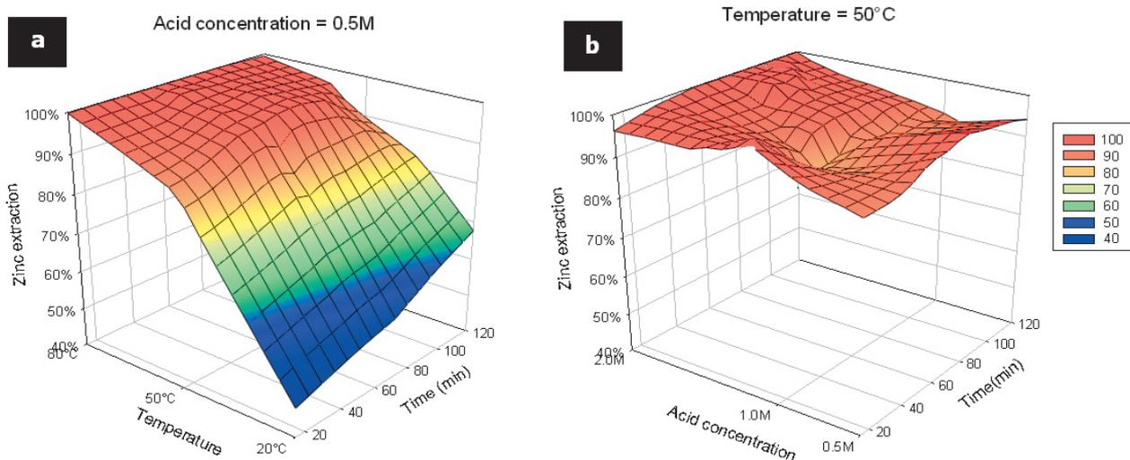
**Fig. 3** Kinetic plots of zinc yielded from temperature (a) and acid concentration (b)
