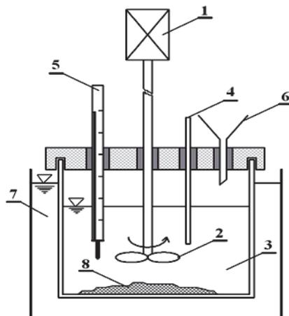
**Fig. 1** Leaching apparatus [11]
