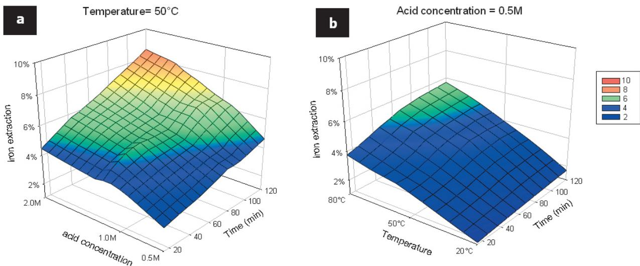
**Fig. 5** Kinetic plots of iron yielded from temperature (a) and acid concentration (b)
