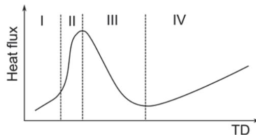
**Fig. 2** Typical boiling curves for water at 0.1 MPa, I - Convection, II - Nucleate boiling, III - Transient boiling, IV - Film boiling
