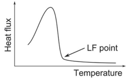
**Fig. 4** Typical shape of the HTC function
