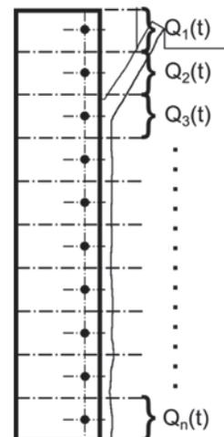
**Fig. 3** Heat flux function allocation to the surface area
