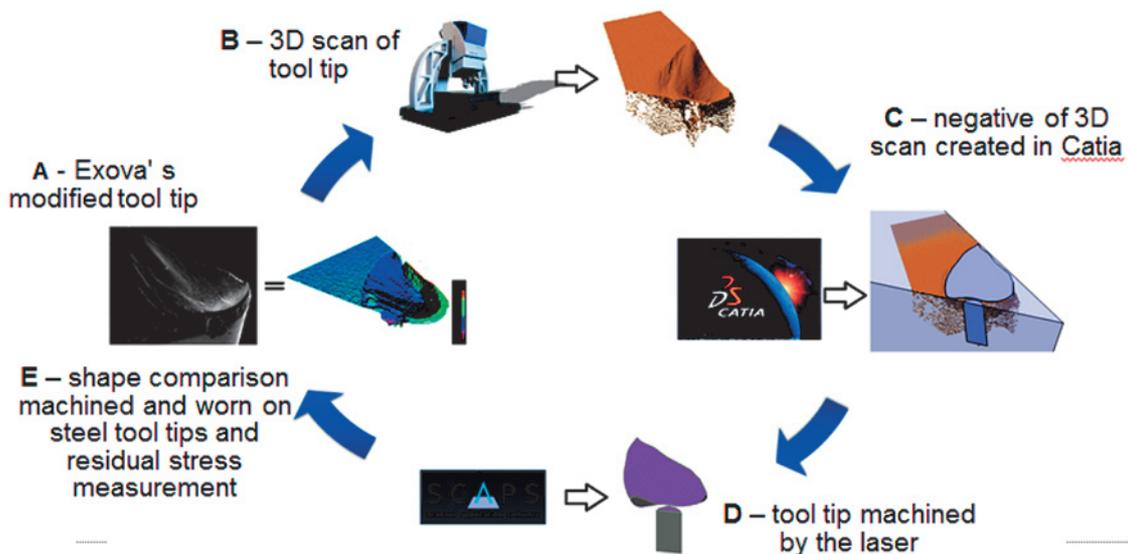
**Fig. 5** Process from the wearing of tool tip, up to laser made tool tip [4]
