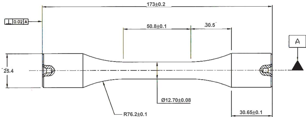
Fig. 1 Test specimen [2]
