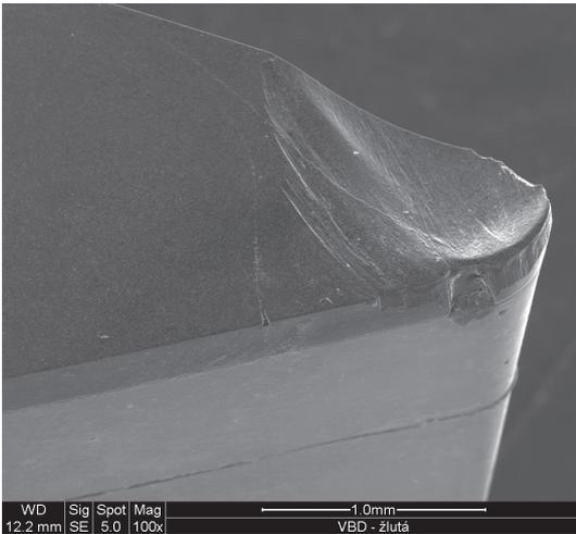
**Fig. 3** Modified diamond tool tip
