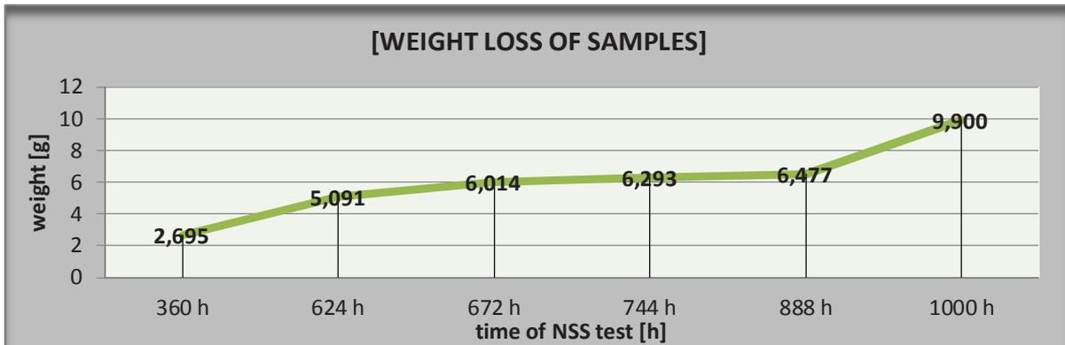
**Fig. 3** Weight change during the corrosion process
