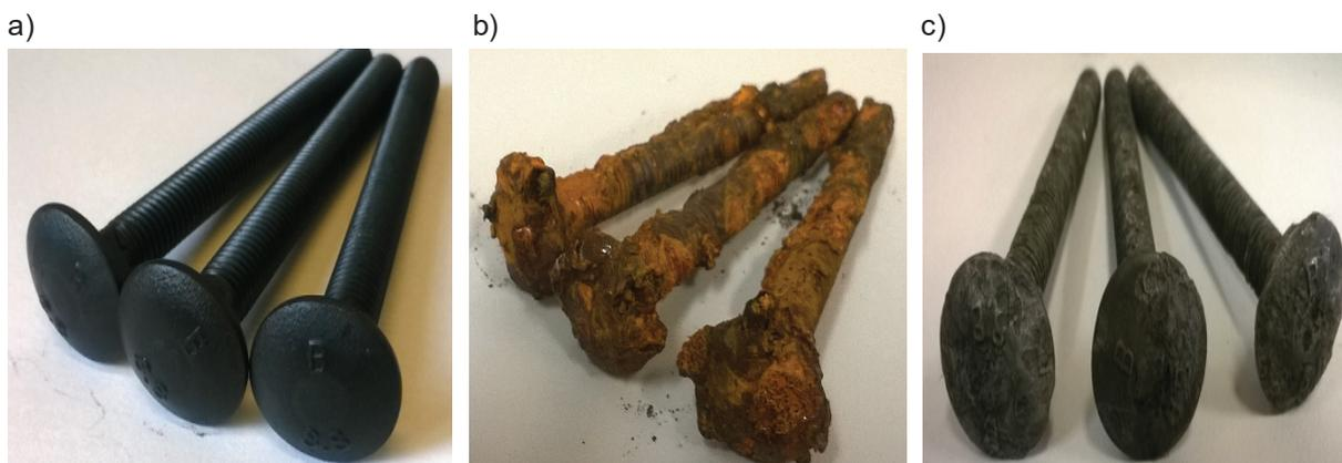
**Fig. 1** The screws M8x80 appearance: a) - before corrosion test, b) - after corrosion test, c)- after cleaning the surface - removal of corrosion products
