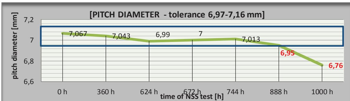
**Fig. 4** Pitch diameter change during the corrosion process
