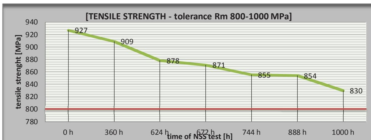
**Fig. 2** Influence of corrosion on the tensile strength change
