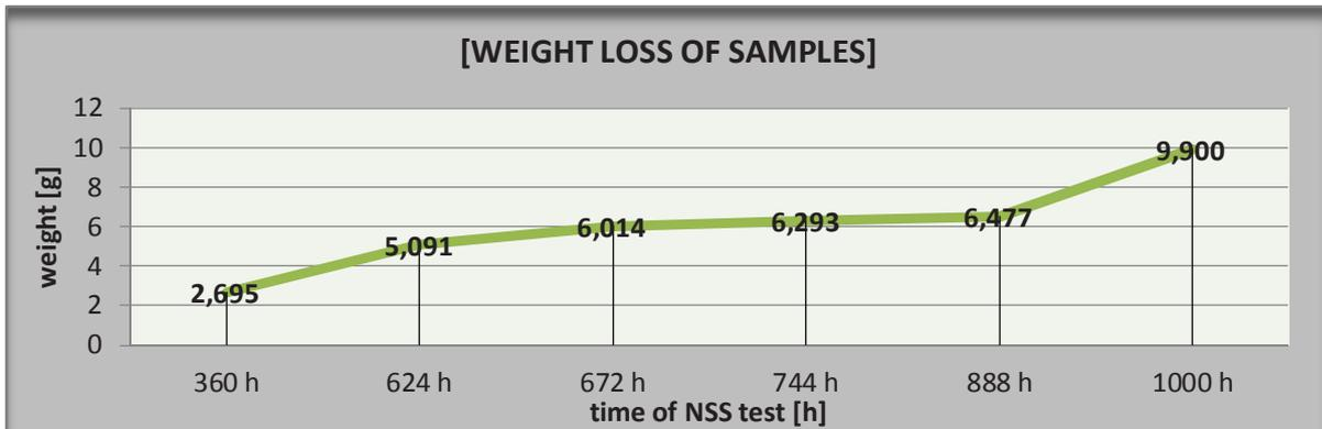
**Fig. 3** Weight change during the corrosion process
