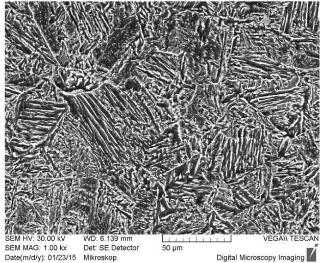
**Fig. 4** Microstructure of unaffected S355N steel
