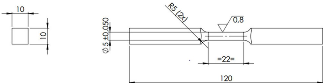
**Fig. 1** The shape of the sample
