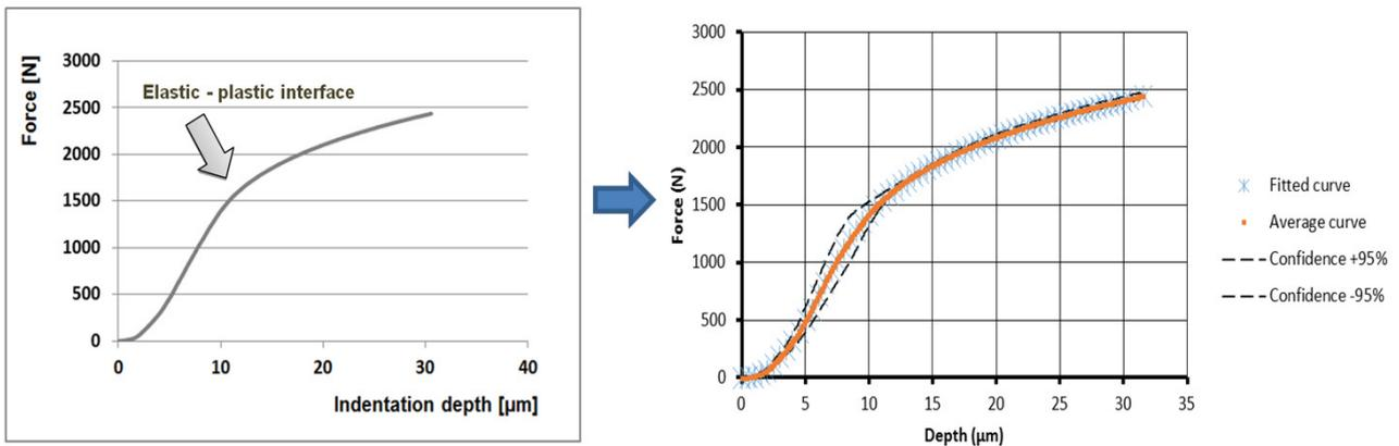
**Fig. 6** Process of indentation method (a), generated values of the the yield strength (b)
