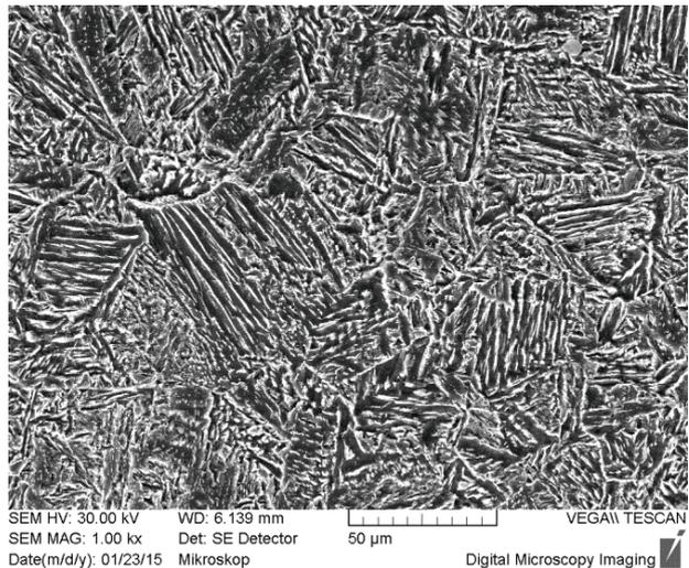
**Fig. 4** Microstructure of unaffected S355N steel
