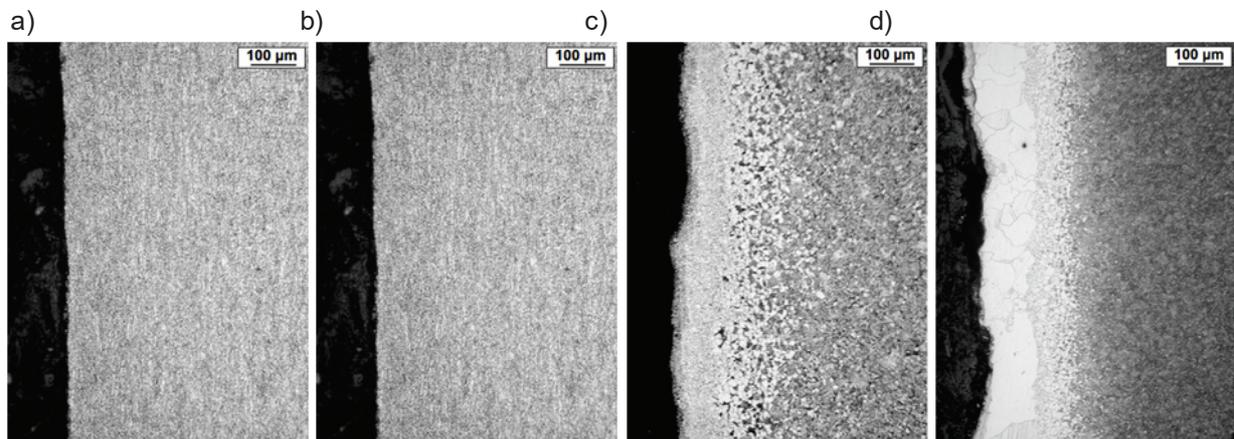
**Fig. 2** Microstructure image of decarburized layer of outer surfaces, a) HT1, b) HT2, c) HT3, d) HT4
