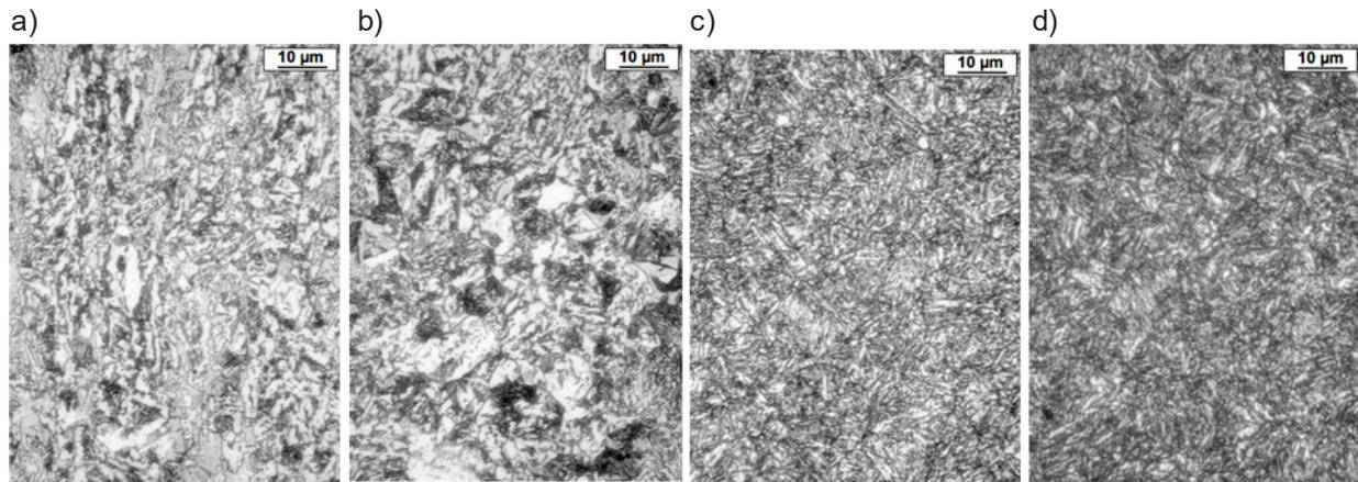
**Fig. 1** Microstructure image of decarburized layer of outer surfaces, a) HT1, b) HT2, c) HT3, d) HT4
