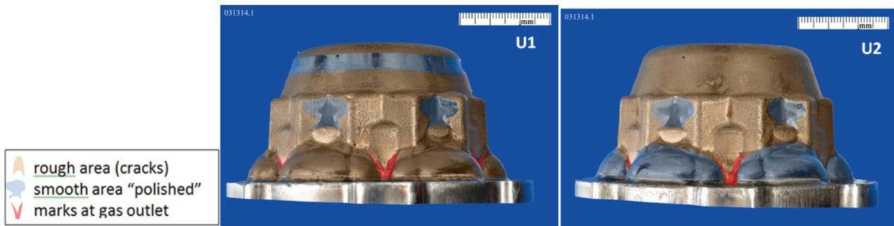
**Fig. 1** Defectology present in the working surfaces
