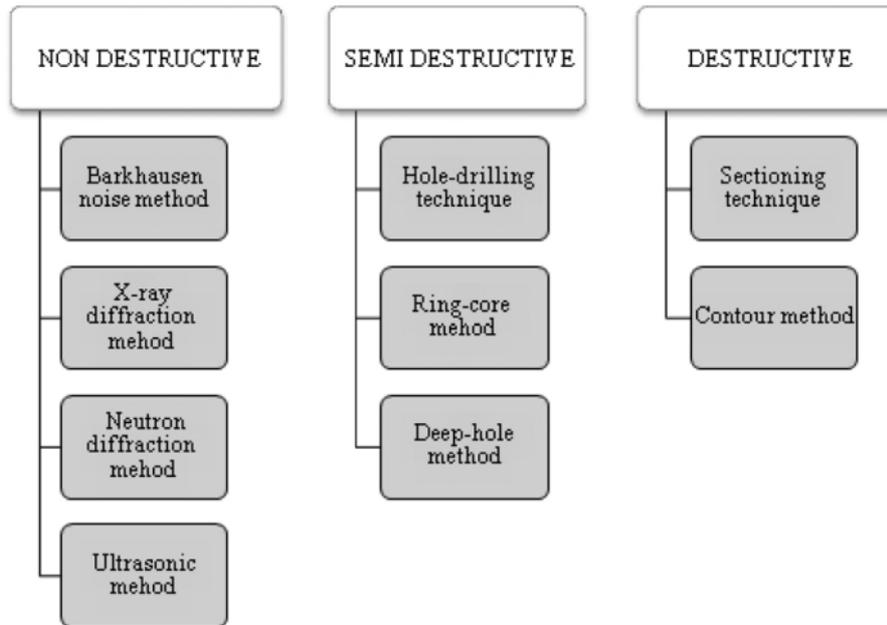
Fig. 1 Residual Stress Measurement Methods [5]
