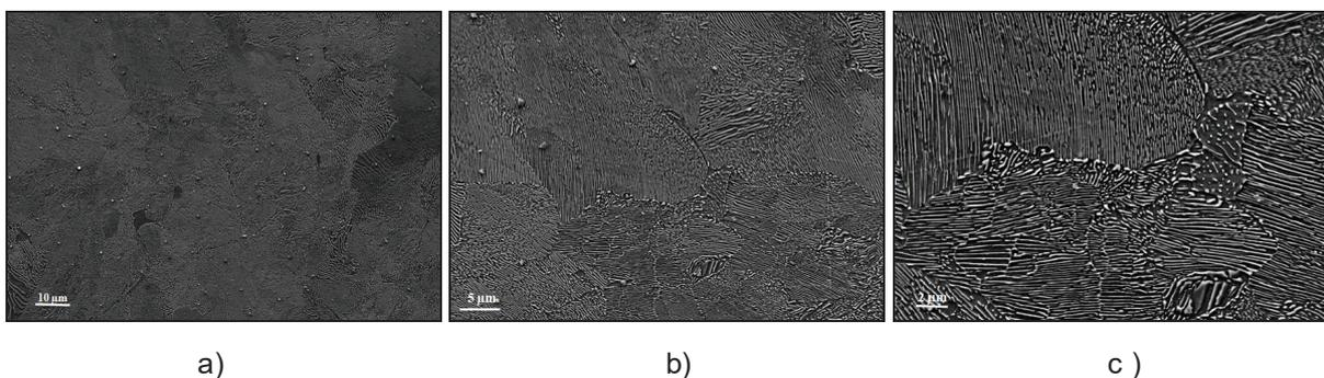
**Fig. 4** SEM images of rail a) 2000X, b) 5000X, c) 10000X
