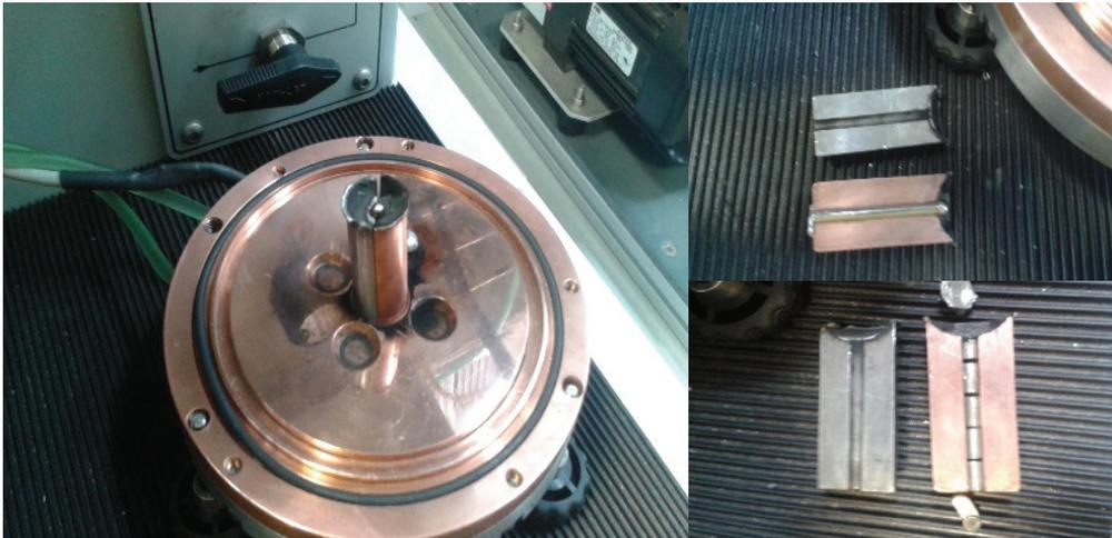
**Fig. 3** Preparation of the ingot by Compact Arc Melter MAM-1
