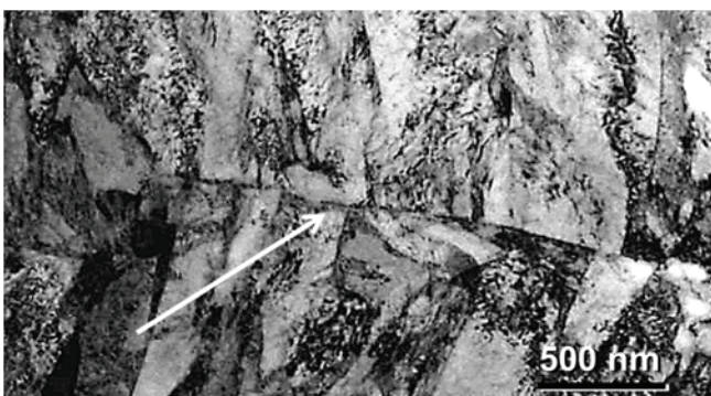
Fig. 5 Prior austenite grain in martensitic matrix, AHSS-3
