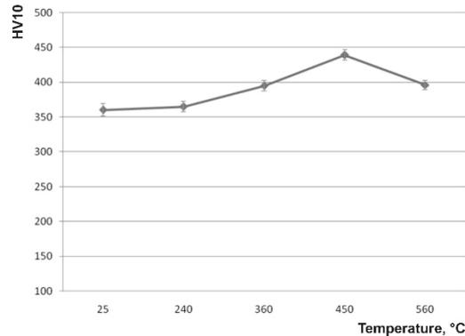
**Fig. 8** Dependence of hardness of samples of investigated steel on the heating temperature after quenching (heating rate 0.05 °C/s)
