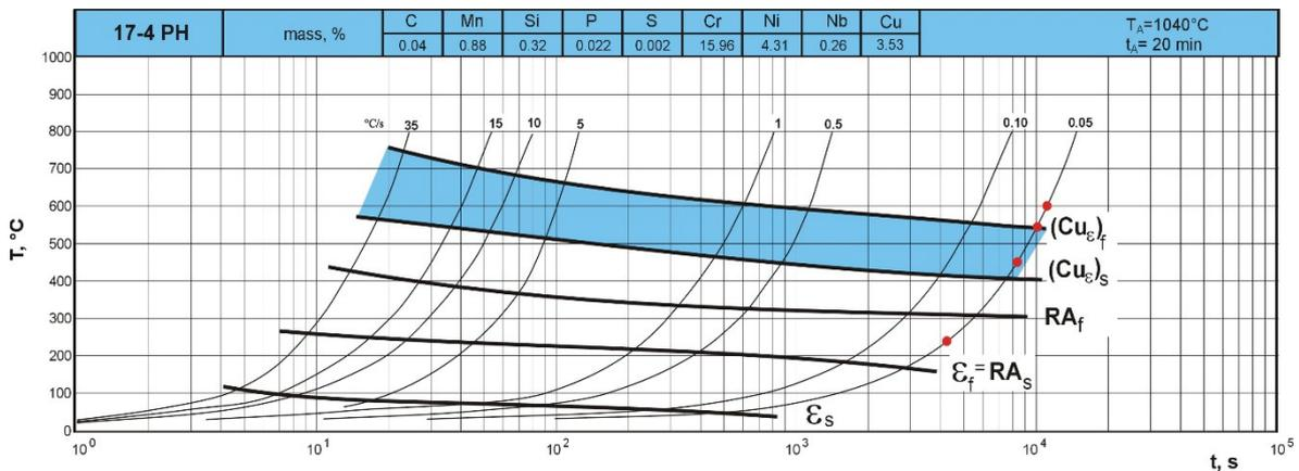
**Fig. 4** CHT diagram for investigated steel. The temperatures of the end of heating the samples for metallographic investigation are marked red
