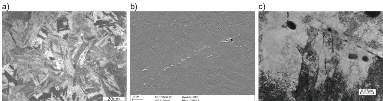
**Fig. 2** Microstructures of the 17-4PH steel after quenching from 1040 °C: a) Light microscope, b) SEM, c) TEM
