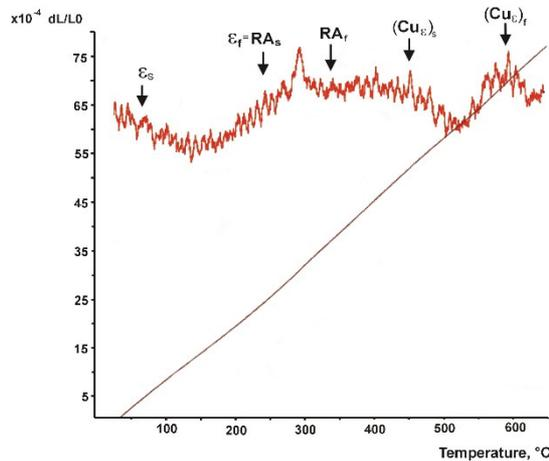
**Fig. 3** The dilatometric curve of heating with the rate of 0.5 °C/s as well as the corresponding differential curve with marked interpretation of phase transformation occurred in the 17-4PH steel during heating from as-quenched state
