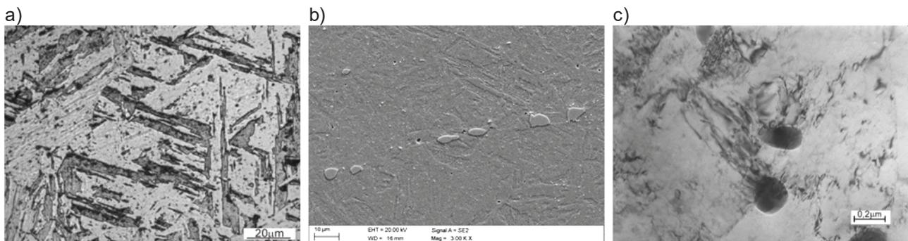
**Fig. 1** Microstructures of the 17-4PH steel in as-delivered condition: a) Light microscope, b) SEM, c) TEM
