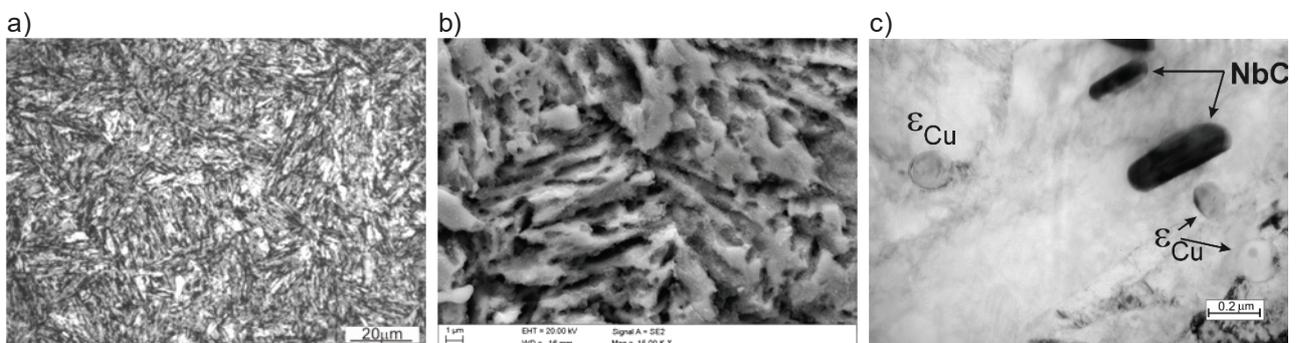
**Fig. 7** The microstructure of investigated 17-4PH steel after quenching from 1040 °C and heated up to 600 °C with the rate of 0.5 °C/s: a) light microscope, b) SEM; c) TEM
