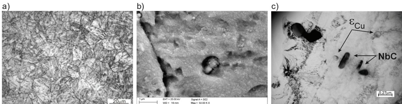
**Fig. 6** The microstructure of investigated 17-4PH steel after quenching from 1040 °C and heated up to 540 °C with the rate of 0.5 °C/s: a) light microscope, b) SEM; c) TEM
