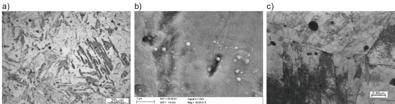
**Fig. 5** The microstructure of investigated 17-4PH steel after quenching from 1040 °C and heated up to 450 °C with the rate of 0.5 °C/s: a) light microscope, b) SEM; c) TEM
