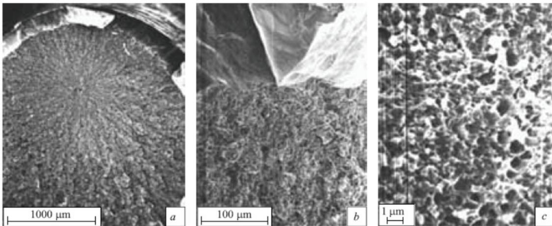
**Fig. 4** Fracture surfaces ( $t_{\text{test}} = -196 \text{ } ^\circ\text{C}$ ) of steel 0.4CCrNi after TMP (variant 3 )
