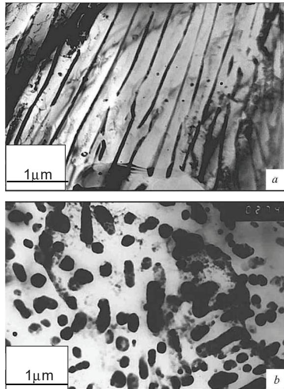
**Fig. 1** Structure of steel 0.4CCrNi after annealing for lamellar (a) and granular (b) pearlite
