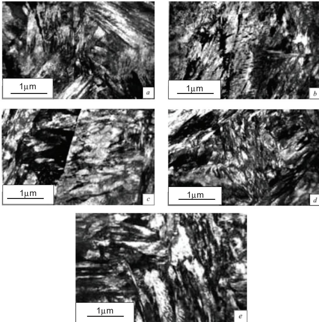
**Fig. 2** Structure of steel 0.4CCrNi after: quenching of non-deformed billets from furnace and induction heating respectively (*a, b*); cold rolling before quenching from induction heating (*c*); cold rolling and annealing respectively at  $500$  and  $600\ ^\circ\text{C}$  before quenching and induction heating (*d, e*)
