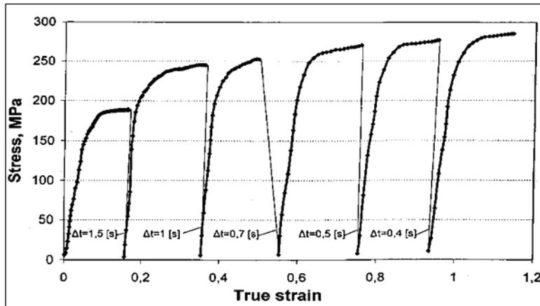
Fig. 5 Simulation of hot rolling using Gleeble 3800 (final temperature 890 °C and strain rate of about 100 s<sup>-1</sup>)
