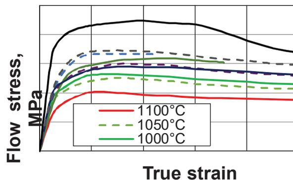
**Fig. 4** Flow stresses for CP steel obtained from torsion tests for various temperatures (in °C) and strain rate equal 2 s<sup>-1</sup>
