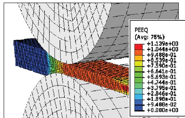
Fig. 7 Effective strain during rolling in first pass
