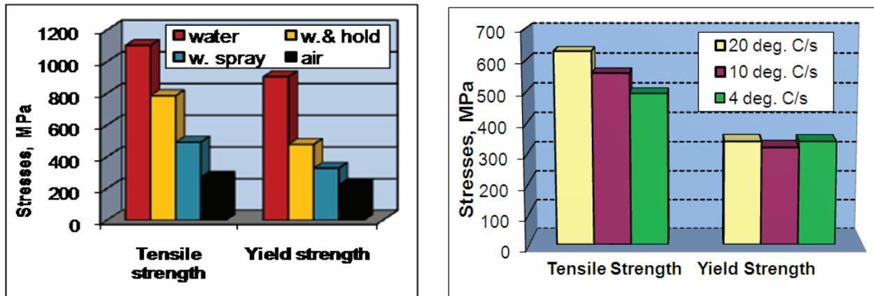
Fig. 10 Tensile strength and yield strength for DP (left) and CP (right) strip samples rolled in three passes
