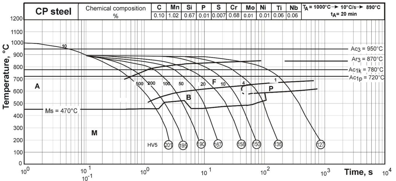
**Fig. 2** Detailed CCT diagram obtained for CP steel
