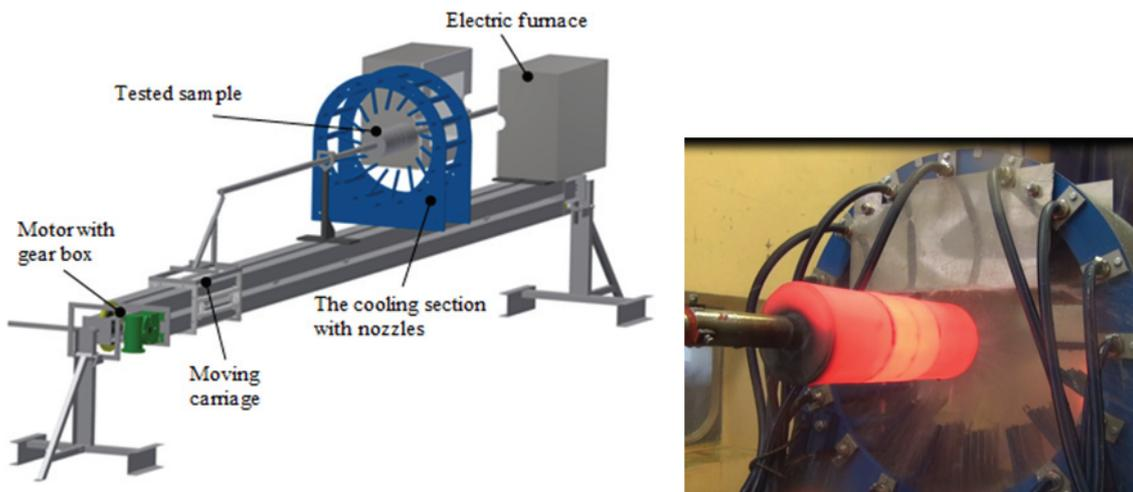
**Fig. 1** Laboratory test bench and a photo of a tube running to the cooling section
