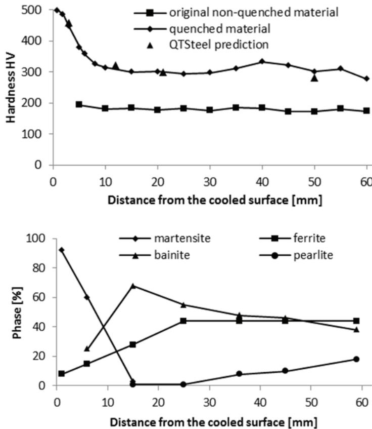
**Fig. 5** Measured hardness (quenched material - HV30, original material - HV 20) and prediction by the QTSteel software [9] (left) and measured microstructure composition (right)
