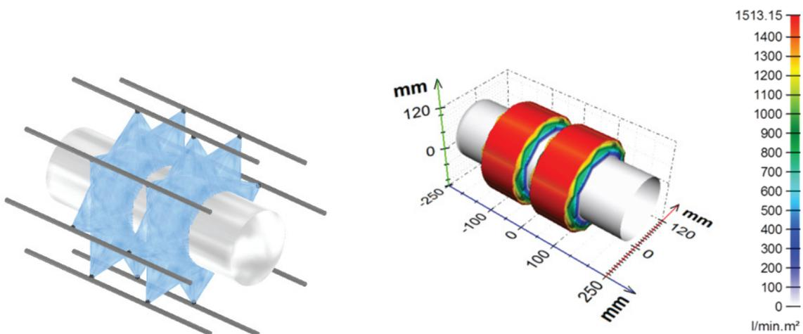
**Fig. 7** Visualization (left) and computed water distribution (right) of the cooling unit used for tube cooling
