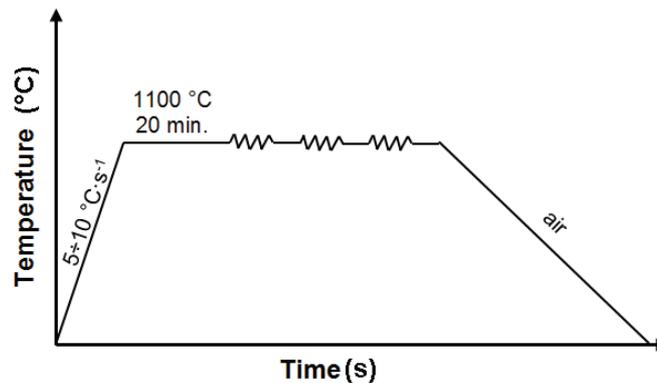
**Fig. 2** Temperature versus time (hot rolling of 1183 sample)
