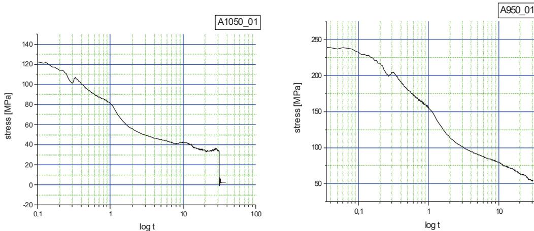
**Fig. 4** Stress-relaxation curves for **A\_1183** (13% Mn at temperature 1050 °C and strain rate 0.1 s<sup>-1</sup>) - left and for **A\_1183** (13% Mn at temperature 950 °C and strain rate 0.1 s<sup>-1</sup>) - right
