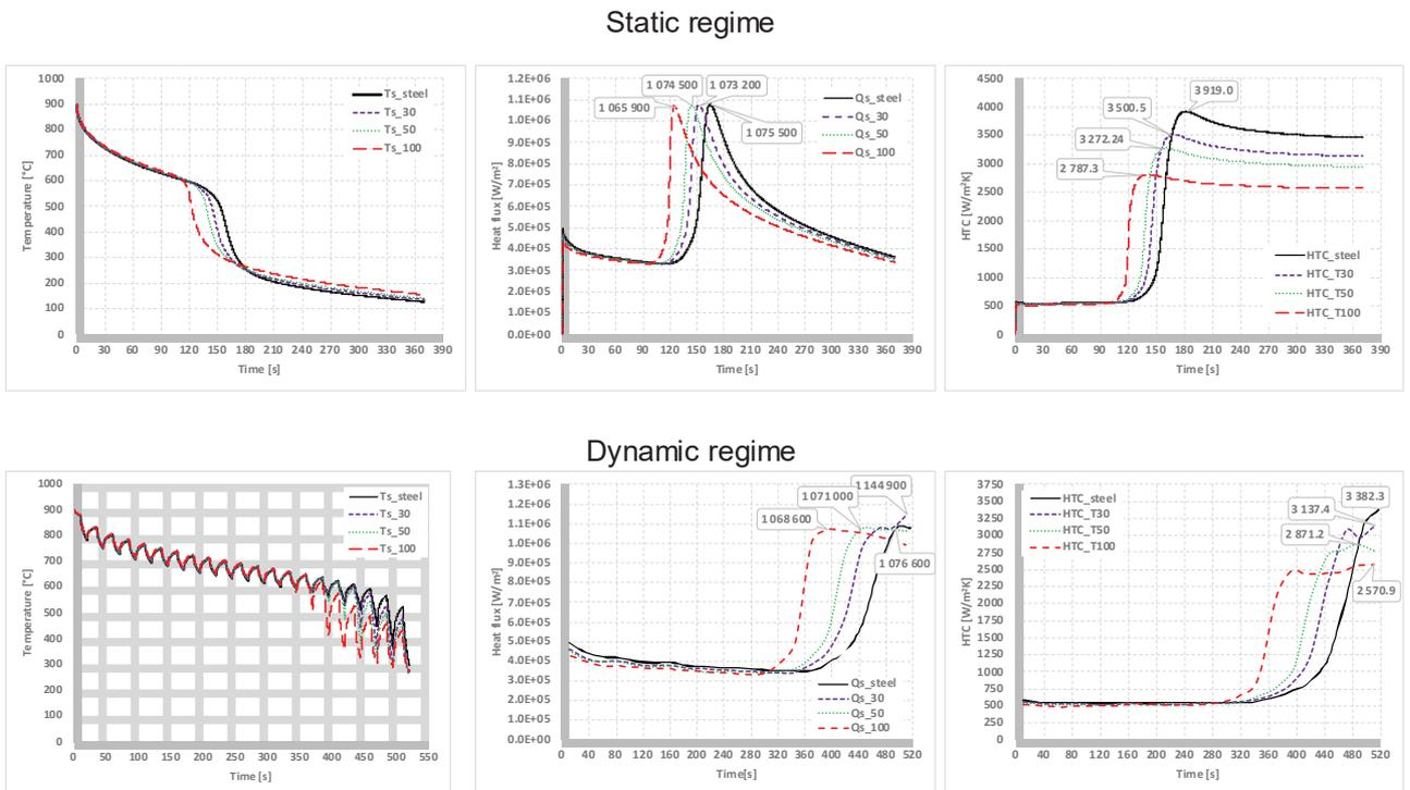
**Fig. 4** Evaluation of the results for thermal conductivity 1.0 W/mK
