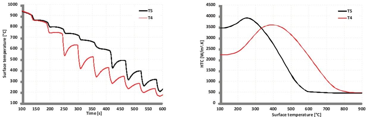
Fig. 1 Measured temperatures in the thermocouples T4 and T5 (left) and heat transfer coefficient (right)
