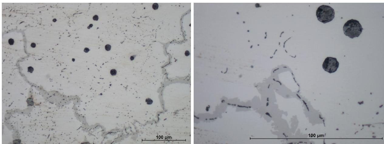
**Fig. 3** Microstructures of silicon cast iron, silicon content 17 %
