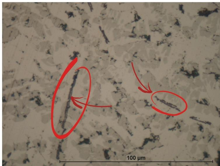
**Fig. 5** Primary precipitates of  $Fe_2Si$  phase, silicon content 19 % [15]
