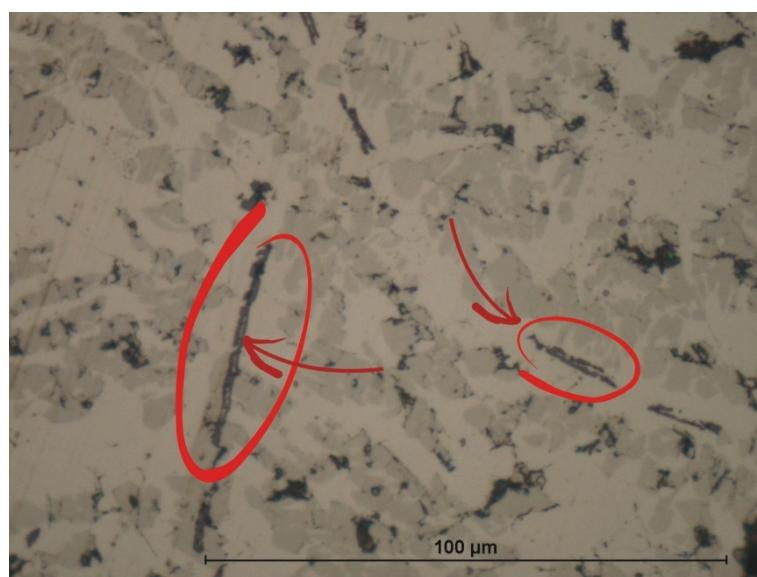
**Fig. 5** Primary precipitates of  $\text{Fe}_2\text{Si}$  phase, silicon content 19 % [15]
