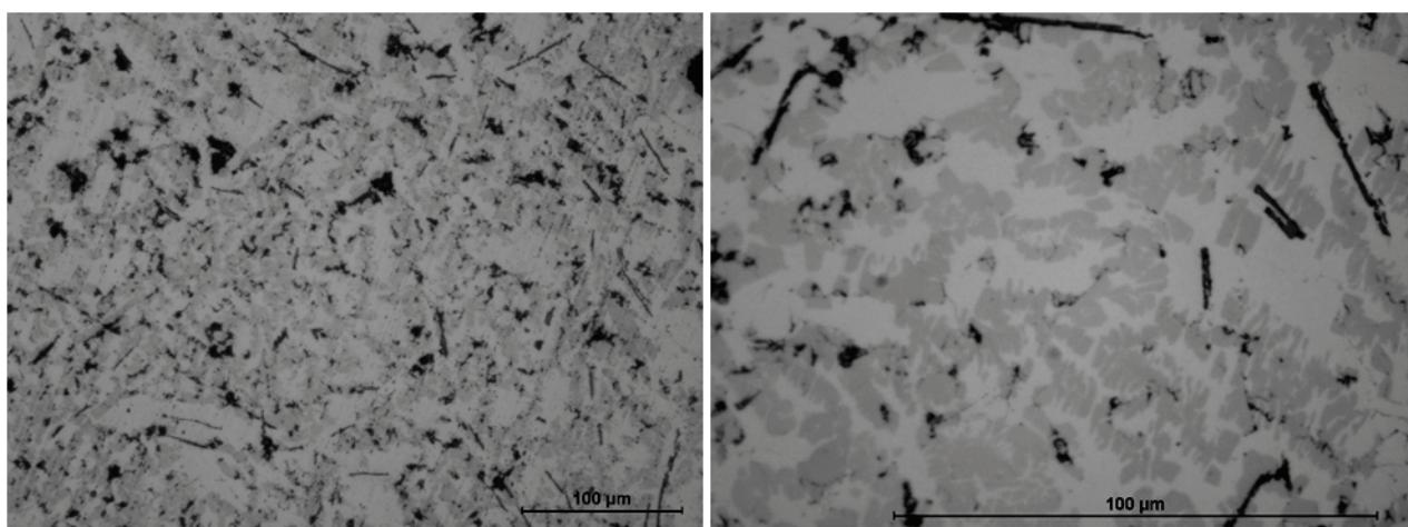
**Fig. 4** Microstructures of silicon cast iron, silicon content 19 %
